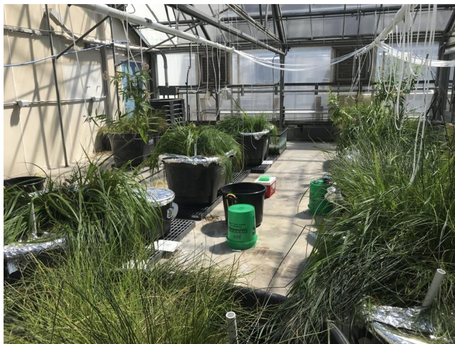
Figure 1: Climate controlled greenhouse with FTW and control mesocosms. Tin foil was placed on mesocosms to limit neonicotinoid degradation via photolysis.
