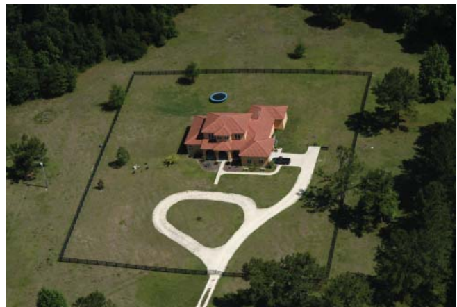
This property has excellent defensible space and would likely be ranked at low risk for wildfire damage by NED2. Credit: Larry Korhnaak.
