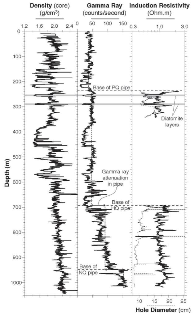
Fig. 4 – Overview of natural gamma radiation, induction resistivity, and calliper (borehole diameter) logs, plotted alongside density measured on core (from Niessen et al. this volume). Natural gamma and density are smoothed with a 20 cm running average. Note that the diatomite layers are well defined in the downhole logs and core physical properties. Natural gamma radiation is attenuated when measured through pipe, but still provides a valid record of formation radioactivity.
