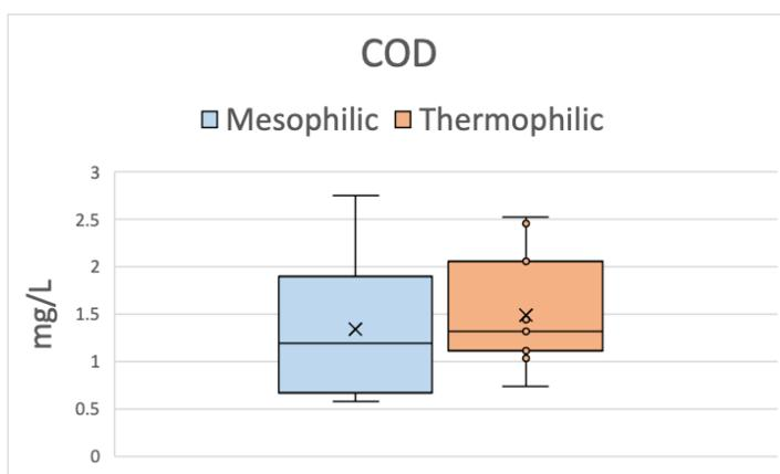
Figure 4.12-Average Chemical Oxygen Demand (COD) in Both the Mesophilic and Thermophilic Columns
