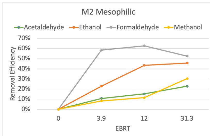
*Figure 4.9-Mixture 2 Removal Efficiency Based on Empty Bed Residence Time Under Mesophilic Conditions*
