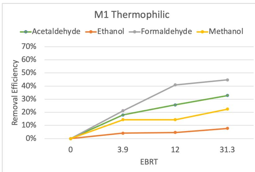
*Figure 4.8-Mixture 1 Removal Efficiency Based on Empty Bed Residence Time Under Thermophilic Conditions*
