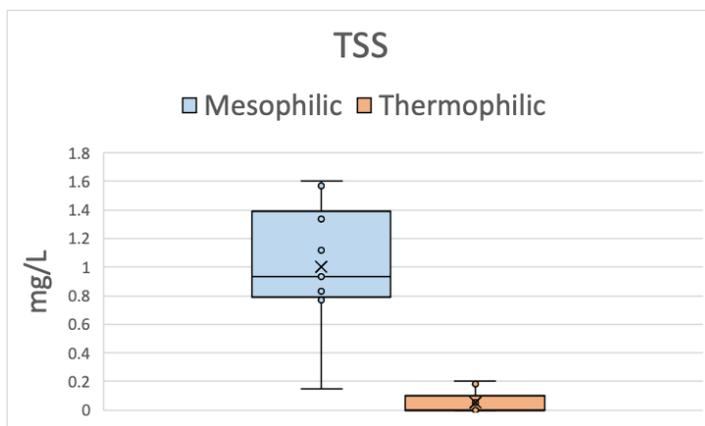
Figure 4.11-Average Total Suspended Solids in Both the Mesophilic and Thermophilic Columns
