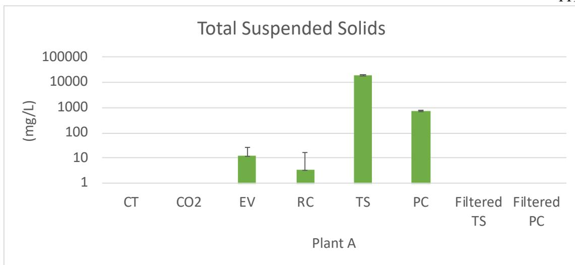
Figure D.5- Total Suspended Solids in Streams From Plant A
