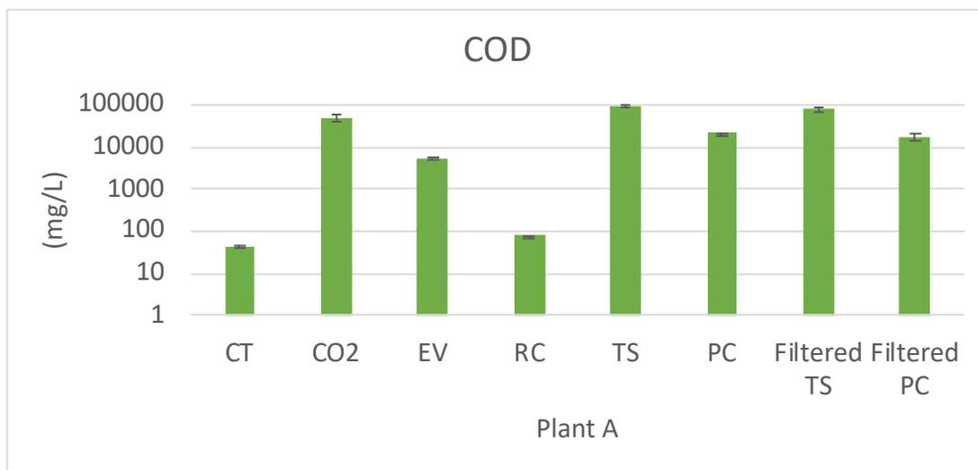
Figure D.1-Chemical Oxygen Demand in Streams From Plant A
