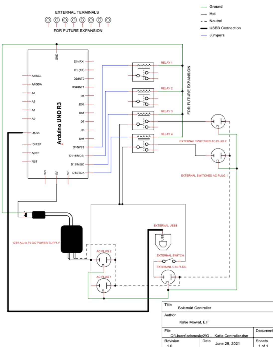
Figure C.1-Schematic of Controller
