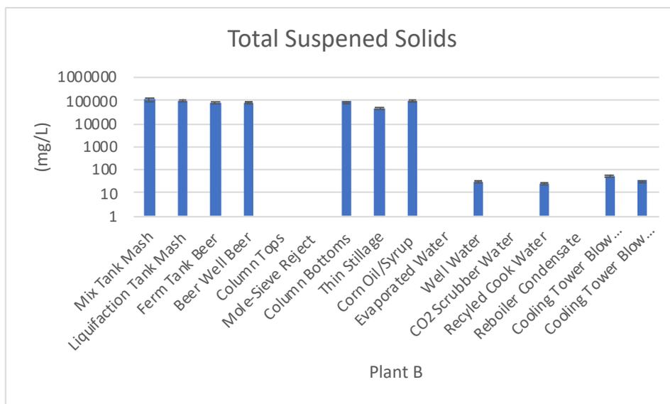
Figure D.10-Total Suspended Solids in Streams From Plant B
