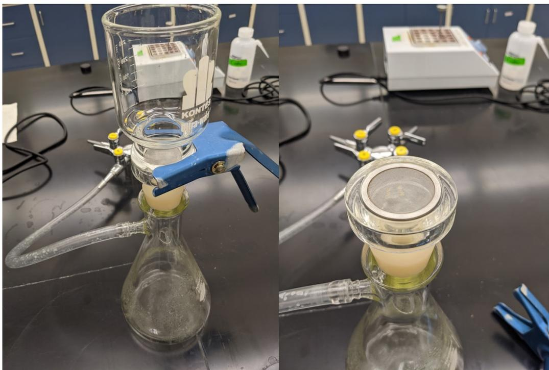
*Figure A.2-Filtration Setup*
