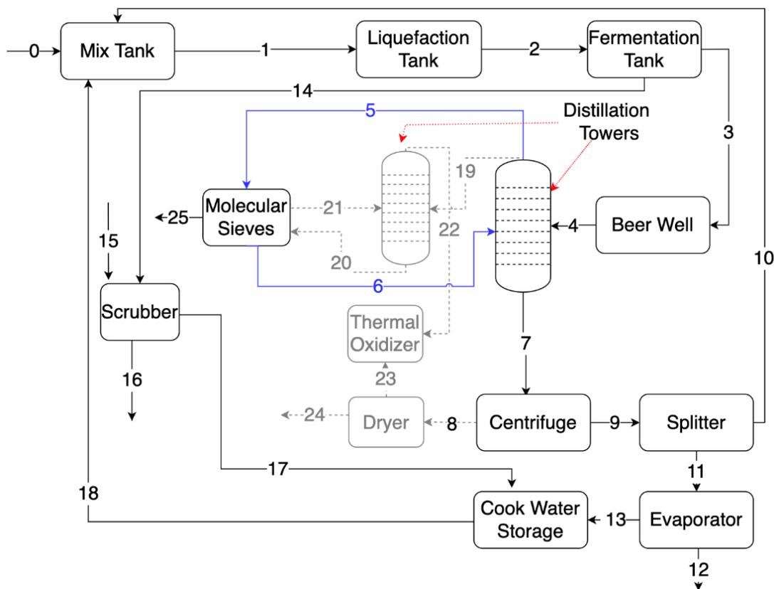
Figure 3.1-Ethanol Plant Flow Diagram with Streams Labeled
