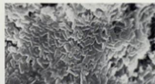
Bacterial cells immobilized on Celite proprietary controlled porosity carrier.
