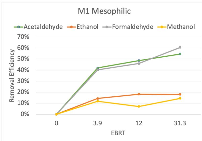
*Figure 4.7-Mixture 1 Removal Efficiency Based on Empty Bed Residence Time Under Mesophilic Conditions*
