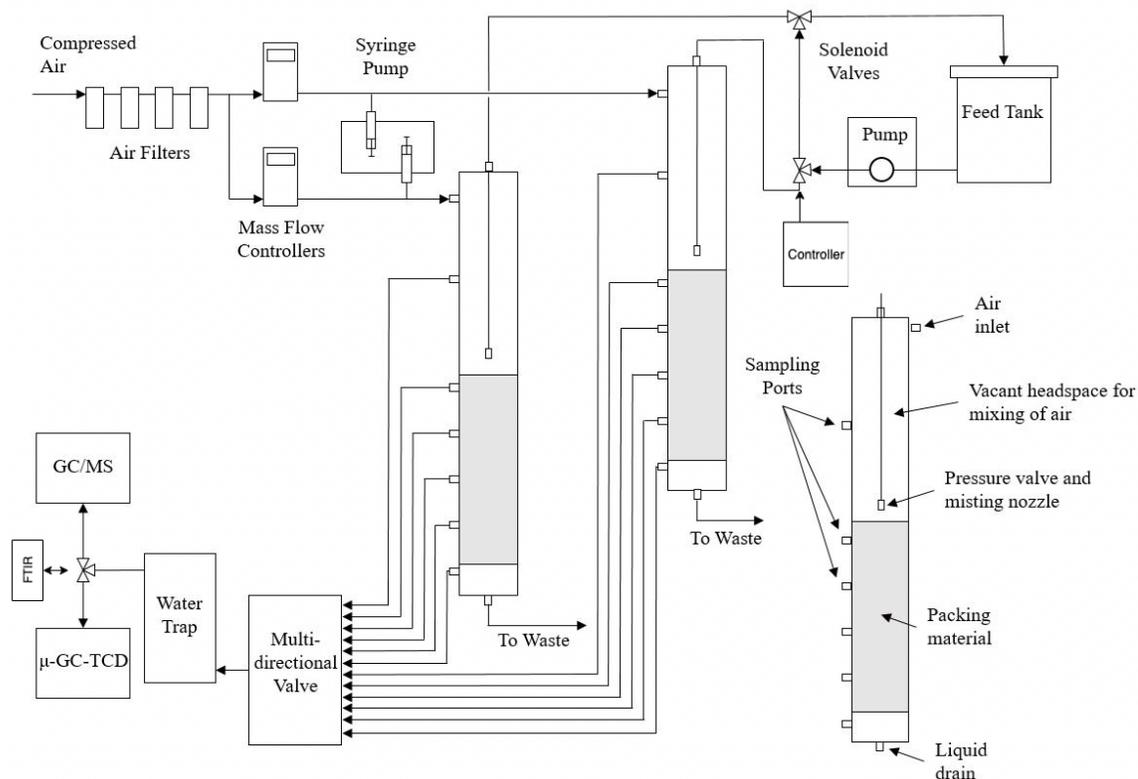
*Figure 3.2-Schematic of Experimental Apparatus*
