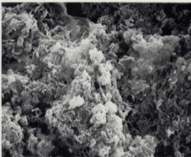
Scanning electron micrograph of typical enzyme carrier pore structure magnification.
