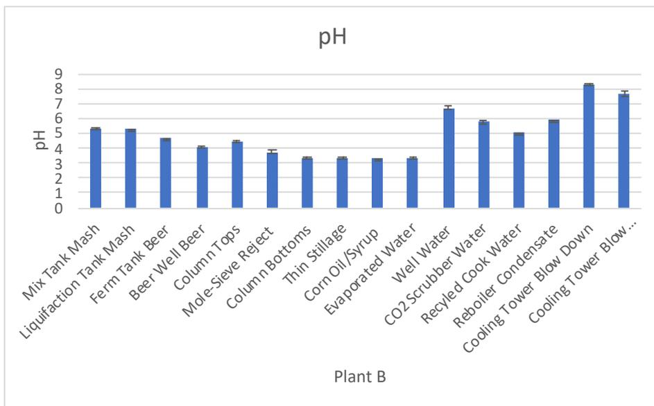
Figure D.9-pH in Streams From Plant B
