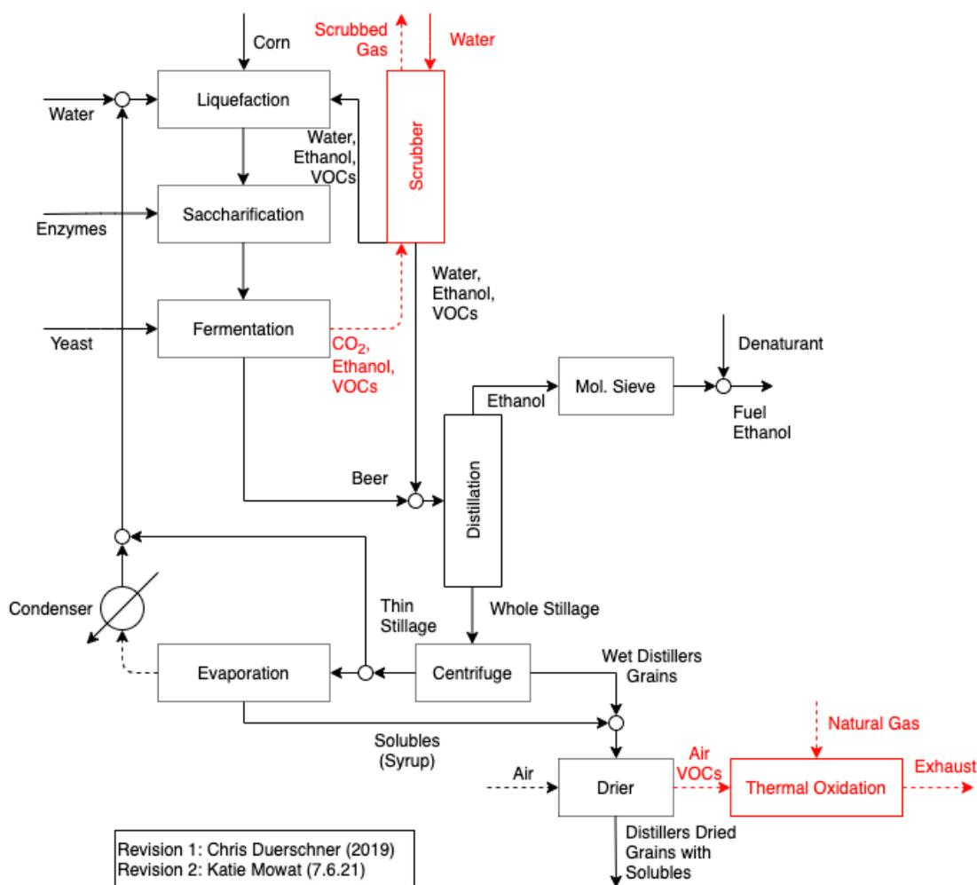
Figure 1.1-Ethanol Plant Flow Diagram (Solid Lines: Liquid, Dashed Lines: Gas)
