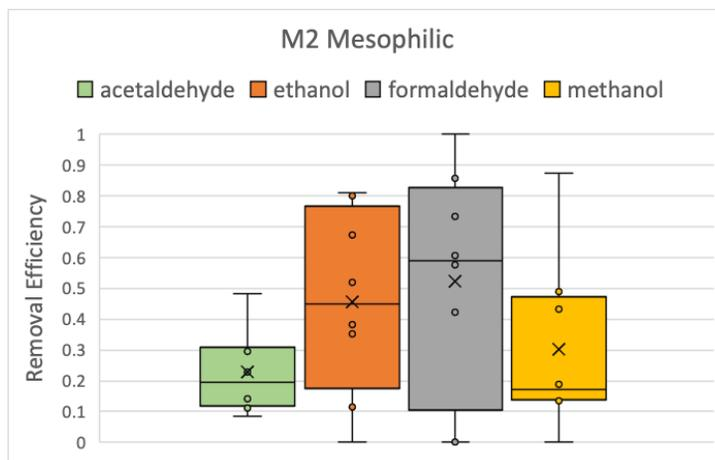
*Figure 4.5-Removal Efficiency of VOCs in Mixture 2 Under Mesophilic Conditions*
