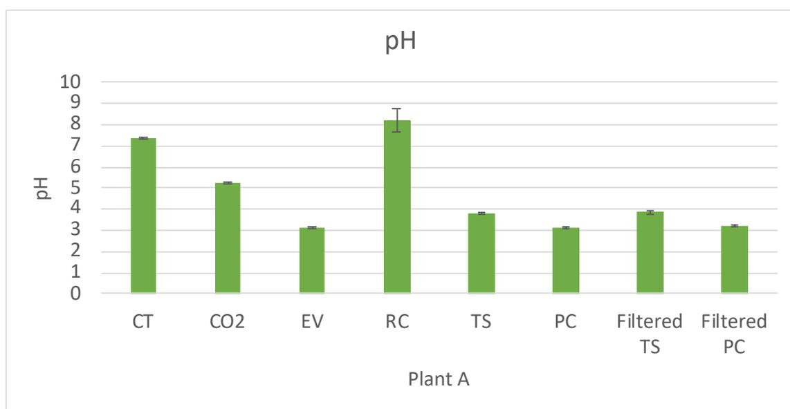
*Figure D.4-pH in Streams From Plant A*
