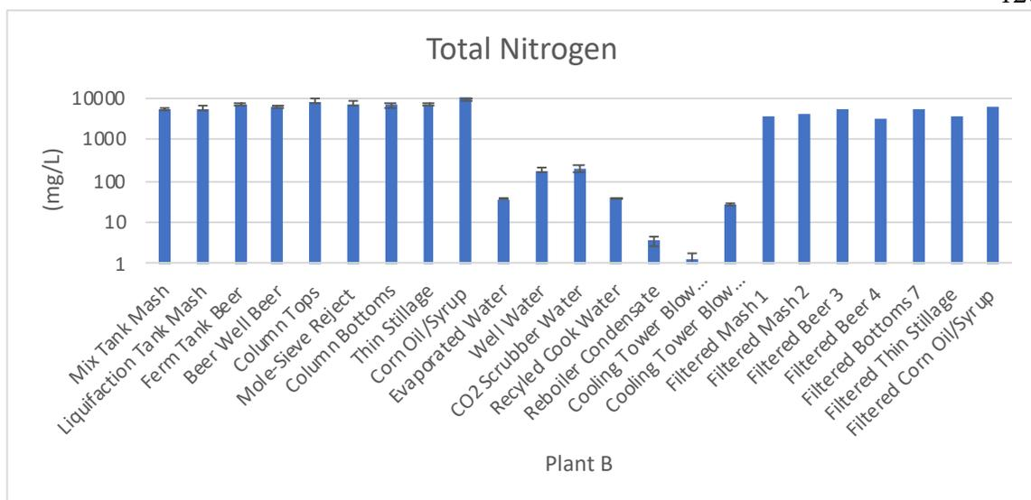
*Figure D.7-Total Nitrogen in Streams From Plant B*
