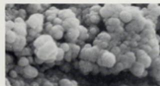
Hybridoma cells immobilized within and on Celite engineered porosity matrix.
