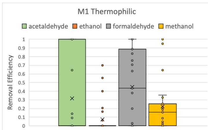
*Figure 4.4-Removal Efficiency of VOCs in Mixture 1 Under Thermophilic Conditions*
