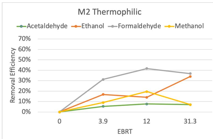
*Figure 4.10-Mixture 2 Removal Efficiency Based on Empty Bed Residence Time Under Thermophilic Condition*
