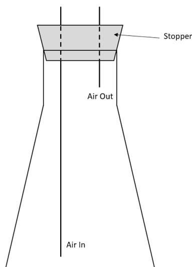
*Figure A.1-Schematic of water trap design used to keep moisture out of the GCMS, GC, and FTIR*
