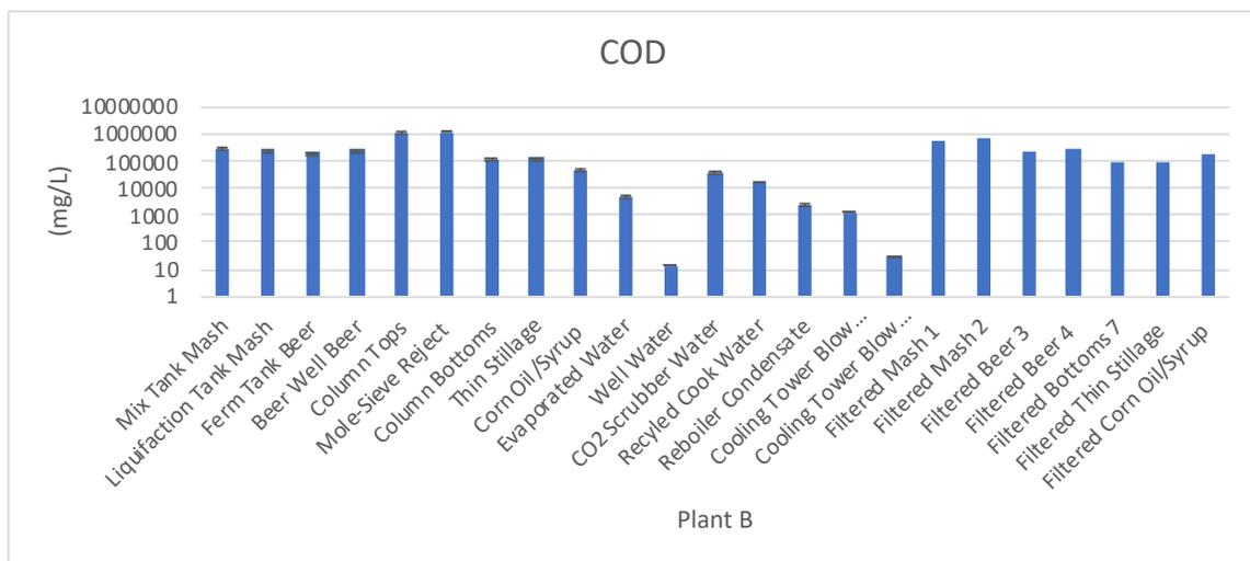
Figure D.6- Chemical Oxygen Demand in Streams From Plant B
