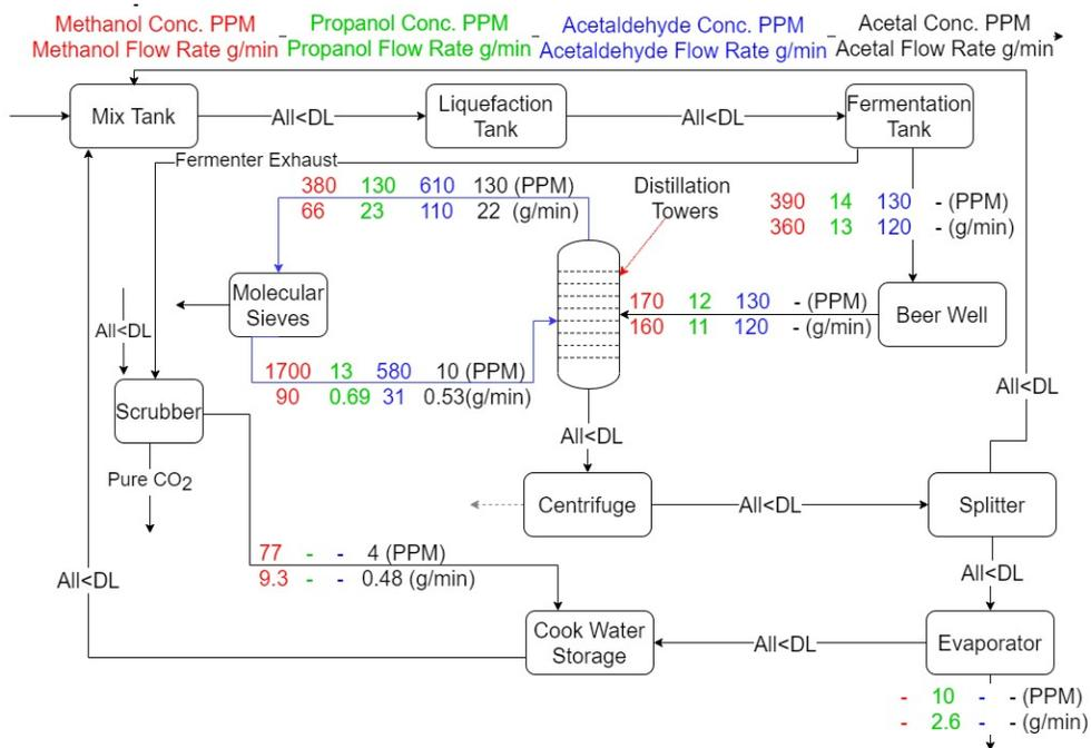
Figure D.11-Plant B Impurities Concentration and Flow Diagram
