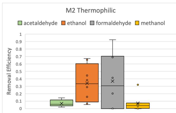
*Figure 4.6-Removal Efficiency of VOCs in Mixture 2 Under Thermophilic Conditions*
