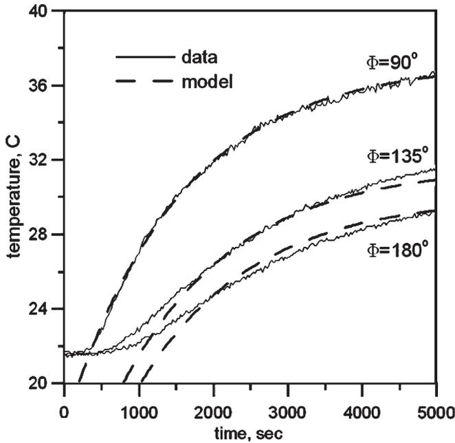
**Figure 6.** Data from thermocouples 6, 7, and 8 for transient heating of a static bearing, and quasi-steady theory at locations  $\phi = 90, 135,$  and  $180$  degrees. The best-fit value of the heat transfer coefficient is  $27.2 \text{ W m}^{-2} \text{ K}^{-1}$ .
