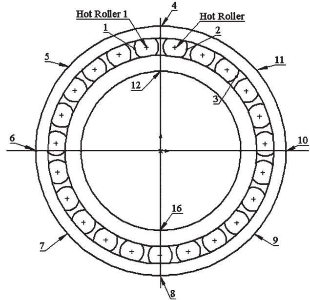
**Figure 5.** Schematic of the railroad roller bearing used for transient heating tests. Thermocouples 4 through 11 are evenly spaced (every 45 degrees) around the outside of the outer bearing race (cup). The two heated rollers are adjacent to thermocouple 4.
