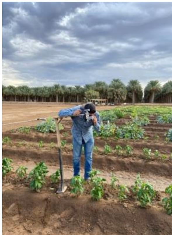
**Figure 1.8.** Using a selfie stick with the camera mounted will ensure taking images at the same height (image by Xinzheng Chen).
