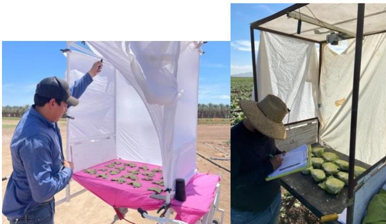
**Figure 1.9.** Using a mobile cart to take images in the field. Taking images for Downy Mildew evaluation on melon leaves (left). Images for quality evaluation of iceberg lettuce for compactness (right). Note camera is mounted to control distance and shade cloth for controlled lighting (image by Xinzheng Chen).
