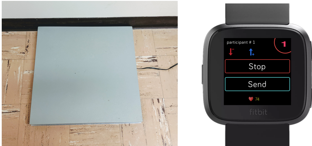
Figure 3.2: An AMTI Force Plate (on the Left) and the Sensor Collector Fitbit App (on the Right)
