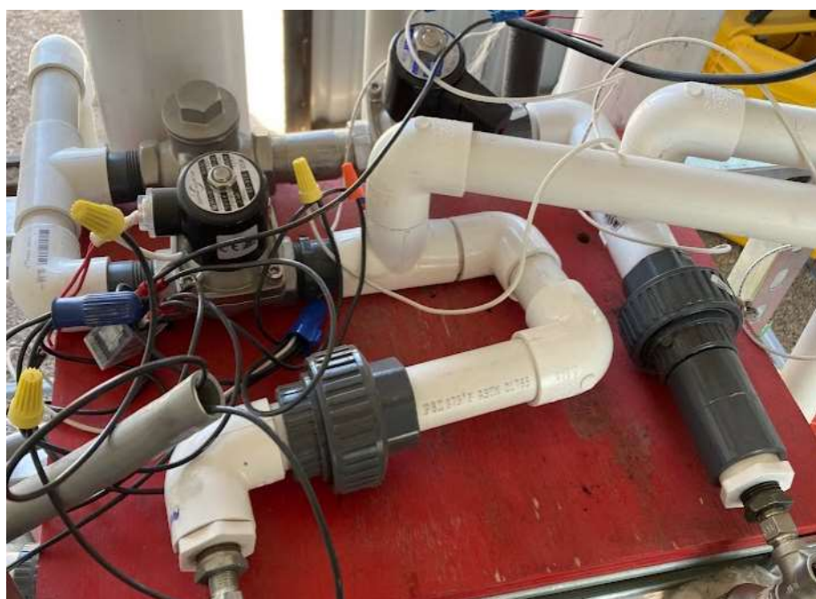
Figure 5.4: Gas Transport System
