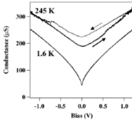
**Figure 1.** Conductance versus bias voltage for a  $\text{CrO}_2/\text{Cr}_2\text{O}_3/\text{CrO}_2$  junction. Asymmetry and hysteresis of the curve are absent at temperatures typically below 20 K, corresponding to the negligible magnetoelectric properties of  $\text{Cr}_2\text{O}_3$ .
