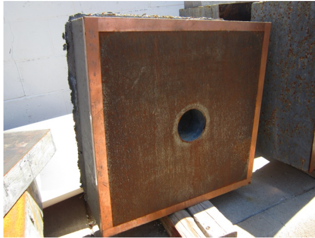
Figure 3-20: Slab with steel plate and domed cavity
