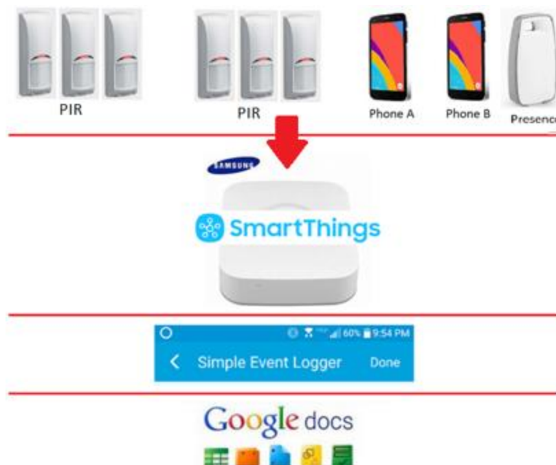
Figure 14: Occupancy detector collection process and device relationship flow.
