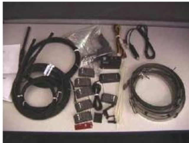
Figure 2.5: Components Kit for Tire-SafeGaurd 10-Tire Rim-Mount TPMS (NHTSA, 2010)
