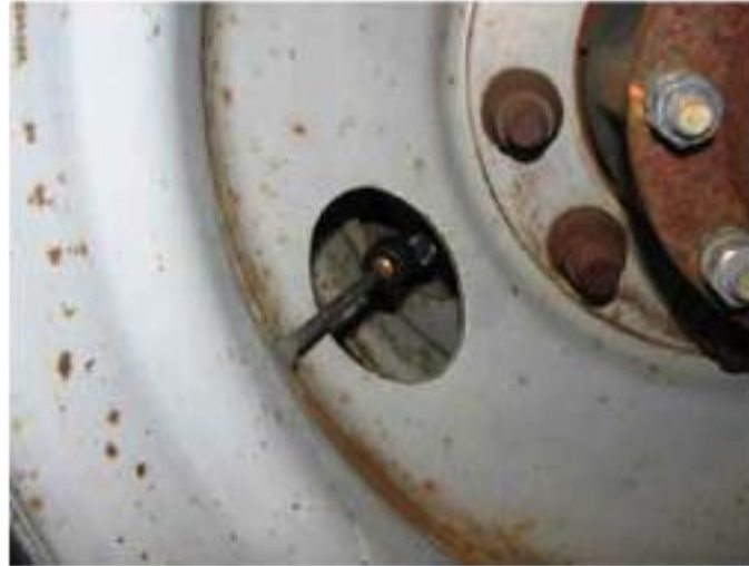
Figure 2.6: Side View of Two PressurePro Sensors mounted on Dual Steel Wheels (NHTSA, 2010).
