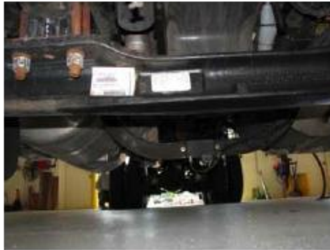
Figure 2.4: SmartWave Receiver/Gateway Mounted on Transmission Lower Crossmember (NHTSA, 2010)
