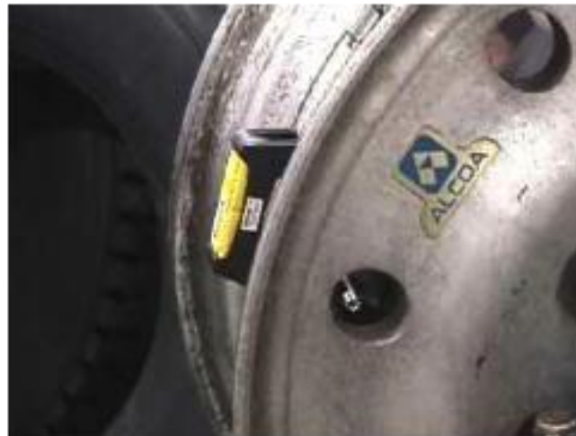
Figure 2.3: SmartWave Sensor Mounted on Lowest Section of Rim with Steel Band (NHTSA, 2010).
