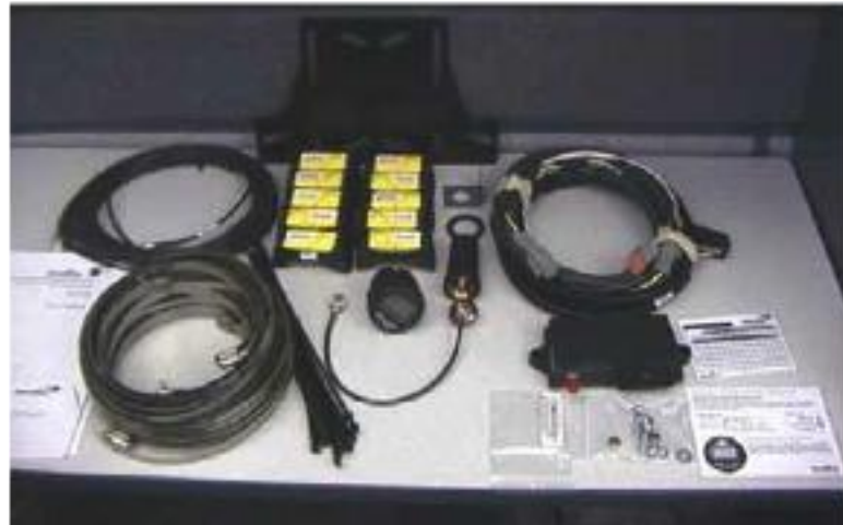
Figure 2.2: Components Kit for SmartWave 10-Tire system (NHTSA, 2010)
