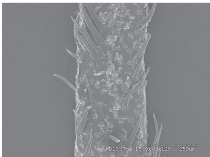
Figure 1. Scanning electron micrograph of an untreated strand mechanically extracted from corn husk.
