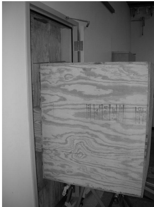
Figure 3.4– Cavity connected to test room and sitting on rollers
