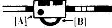
Passenger and freight station (first class, with water tower [A] and depot [B])
