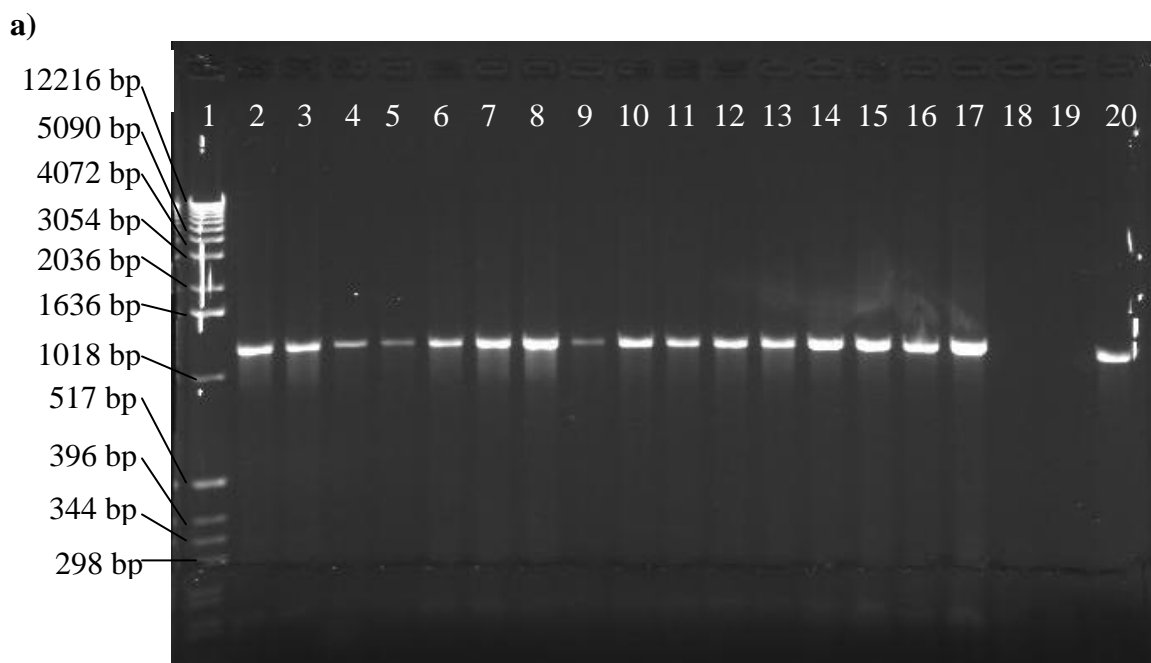
a) RT-PCR Products from Plants Testing Positive for Systemic Infection by PS81 – Gel of 20 positive samples of Taq -PCR products that were purified using a PCR Purification Kit to be sequenced. Lane 1 is 1 Kb ladder, lanes 2-20 purified PCR positive PS81 samples. Four samples were taken for each set of PS81. A positive is ~1,200 nt band
