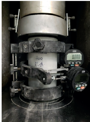
Figure 4.8. Modulus of Elasticity Test Setup.
