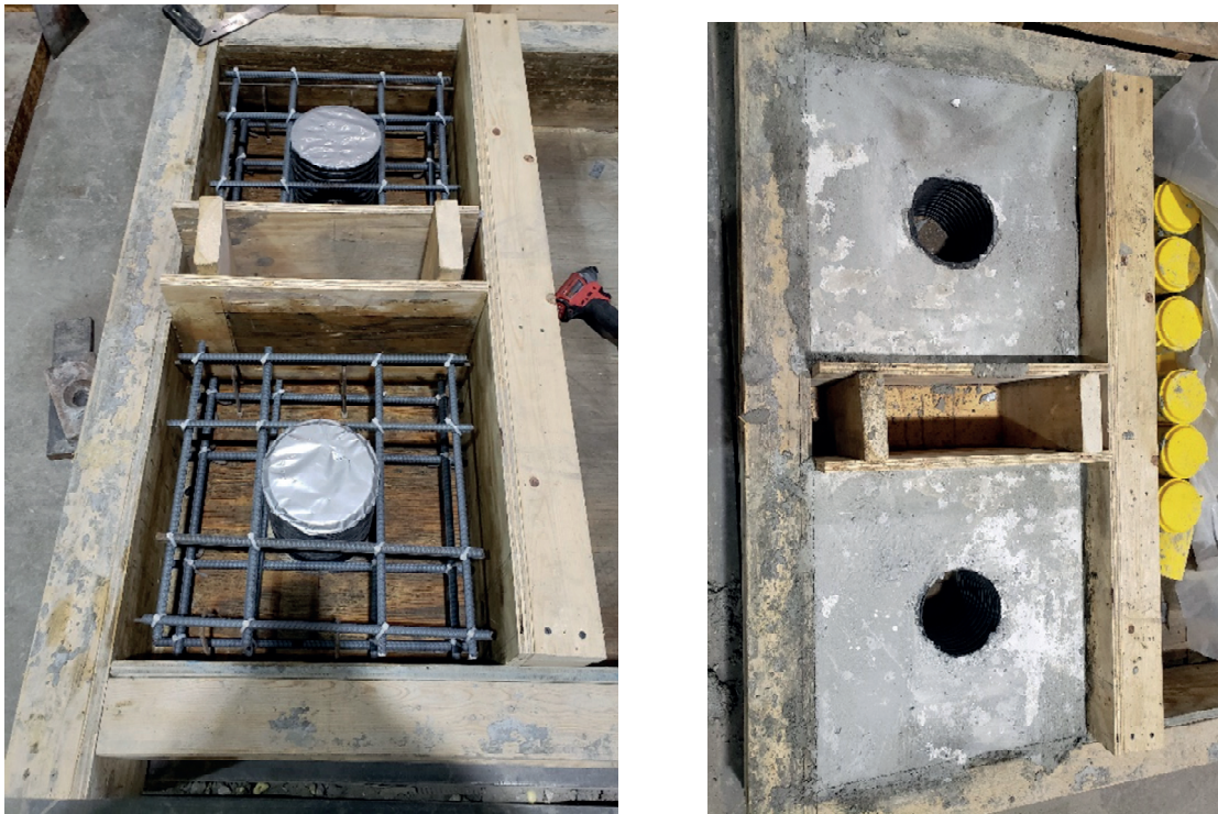
Figure 6.11. Concrete Section of Double Shear Test Specimen.
