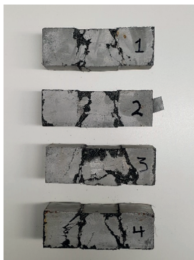
Figure 6.2. Double Shear Failure Mode of Direct Shear Test Specimen.
