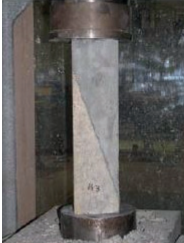
Figure 2.13. Slant Shear Test Configuration (Carbonell Muñoz 2012).
