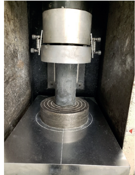
Figure 4.3. Cylinder End Grinding and Testing
