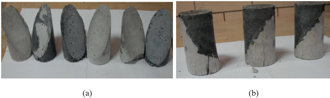
Figure 2.7. Failure Modes; (a) Failure along Interface Plane, (b) Normal Concrete Failure (Harris et al. 2011)
