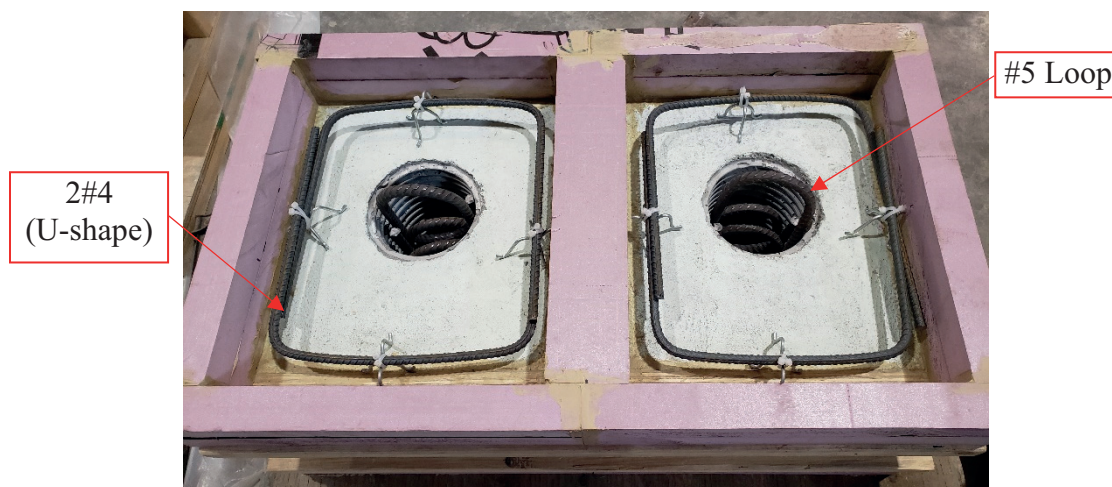
Figure 6.13. Double Shear Specimen Forming
