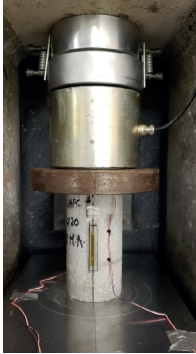
Figure 4.11. Test Setup for Obtaining Stress-Strain Behavior.
