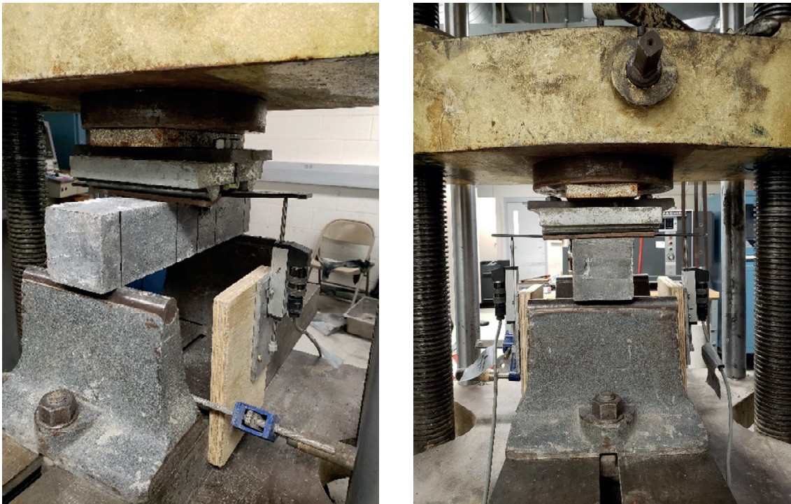
Figure 4.13. Flexure Strength Test Setup.
