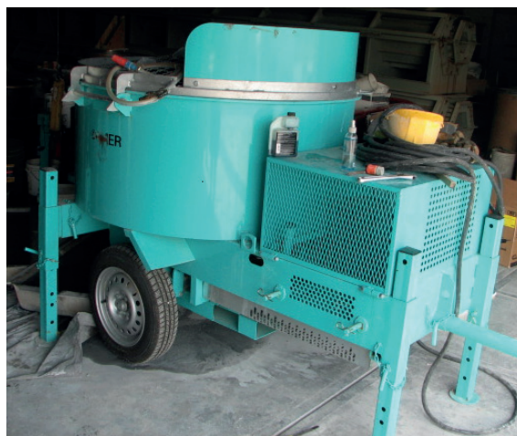
Figure 4.2. Mortar Mixer Used for Mixing UHPC
