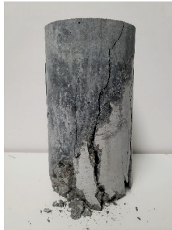
Figure 5.9. Failure Mode for Slant Shear Specimens Using UHPC without Fibers.
