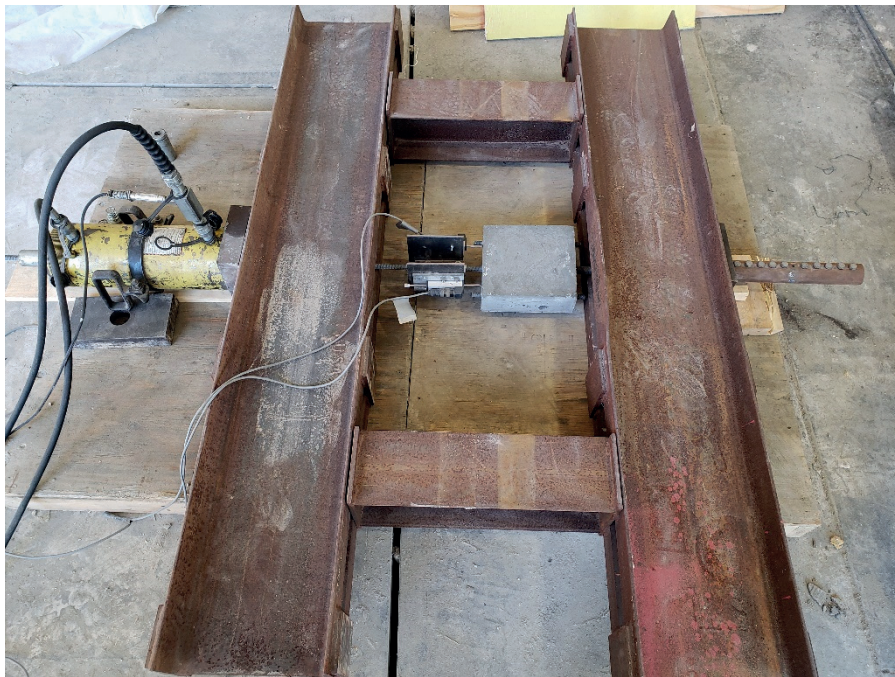
Figure 4.22. Rebar Pullout Test Setup of UHPC 1900 Mix.
