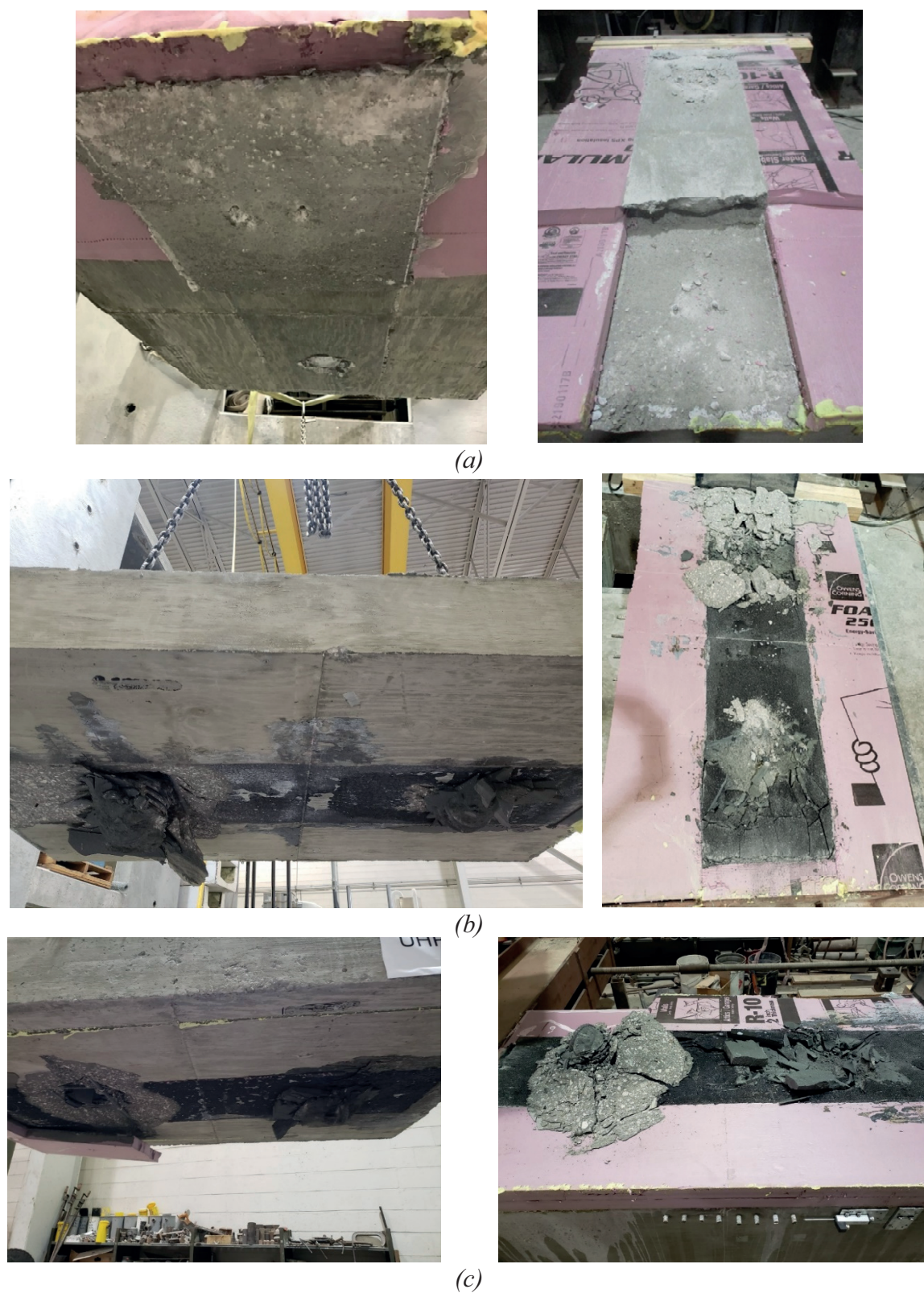
Figure 6.40. Full-Scale Specimen Failure Modes; (a)UHPC#1, (b)UHPC#2, and (c)UHPC#3.
