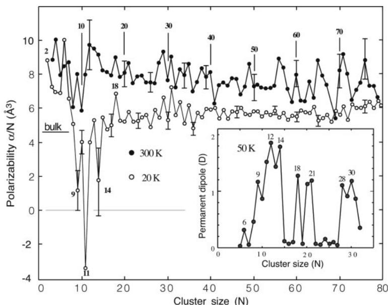
80 kV/cm and 300 K is 0.031 D, whereas the permanent dipole moment associated with the tail extends to 1.8 D. The large disparity in these moments, and thus the large disparity in the deflections, allows the two components to be resolved even at relatively low fields.
