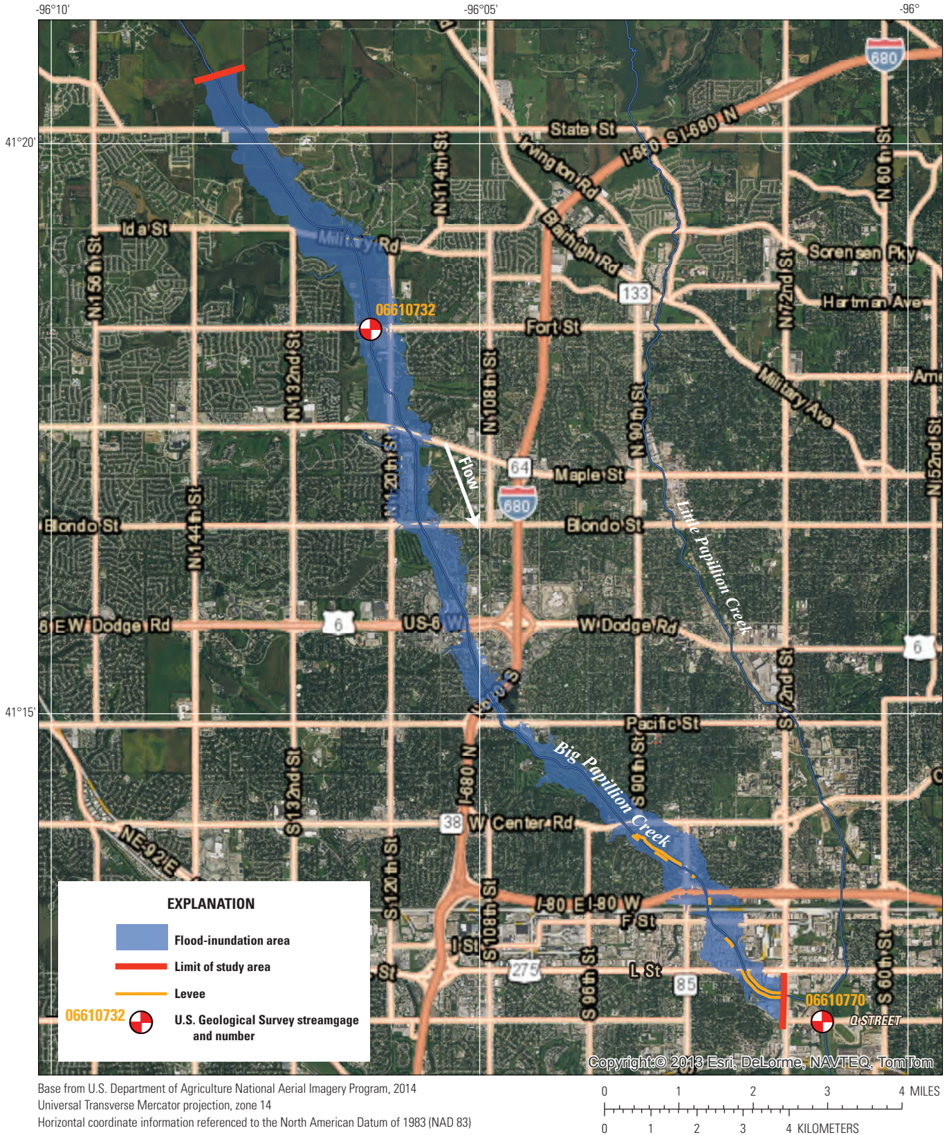
Figure 2. Flood-inundation map for the Big Papillion Creek at Fort Street at Omaha, Nebraska, corresponding to a stage of 32.00 feet at the U.S. Geological Survey streamgage (station 06610732).
