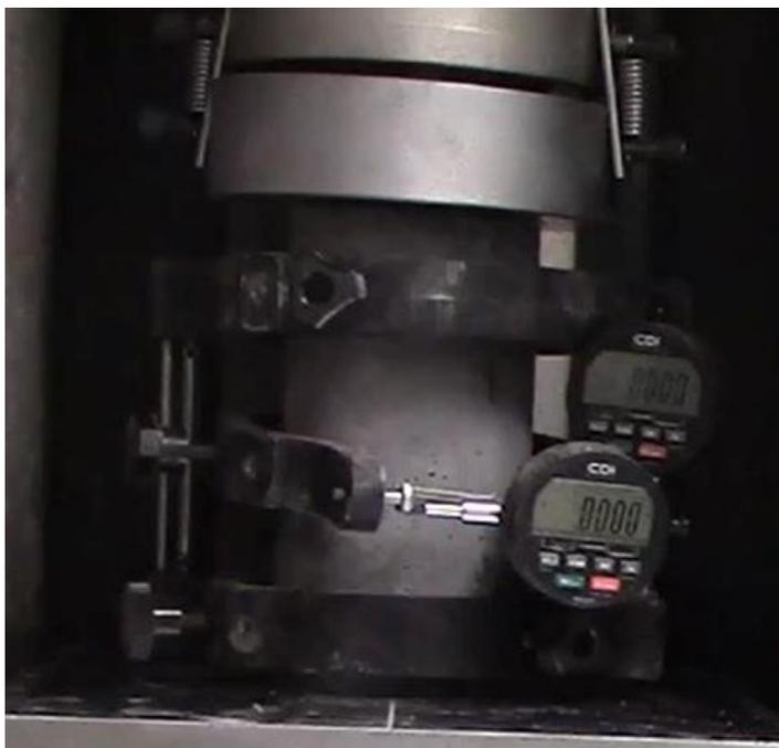
Figure 58: Extensometer cage installed on a UHPC cylinder for the modulus of elasticity testing
