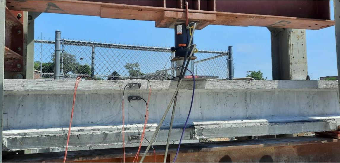
Figure 111: Strengthened beam #1 test setup and instrumentation
