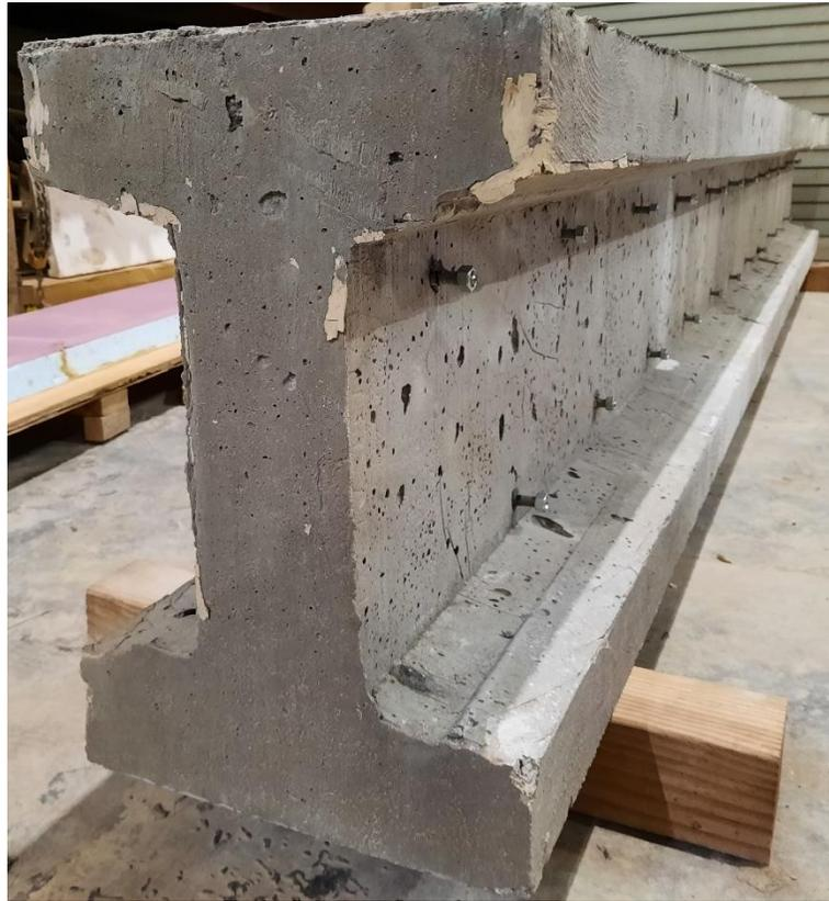
Figure 132: Shear strengthening procedure, steps 1 and 2: roughening of the interface and installing anchors
