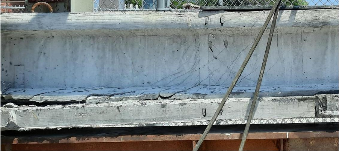
Figure 114: Strengthened beam #1 failure mode
