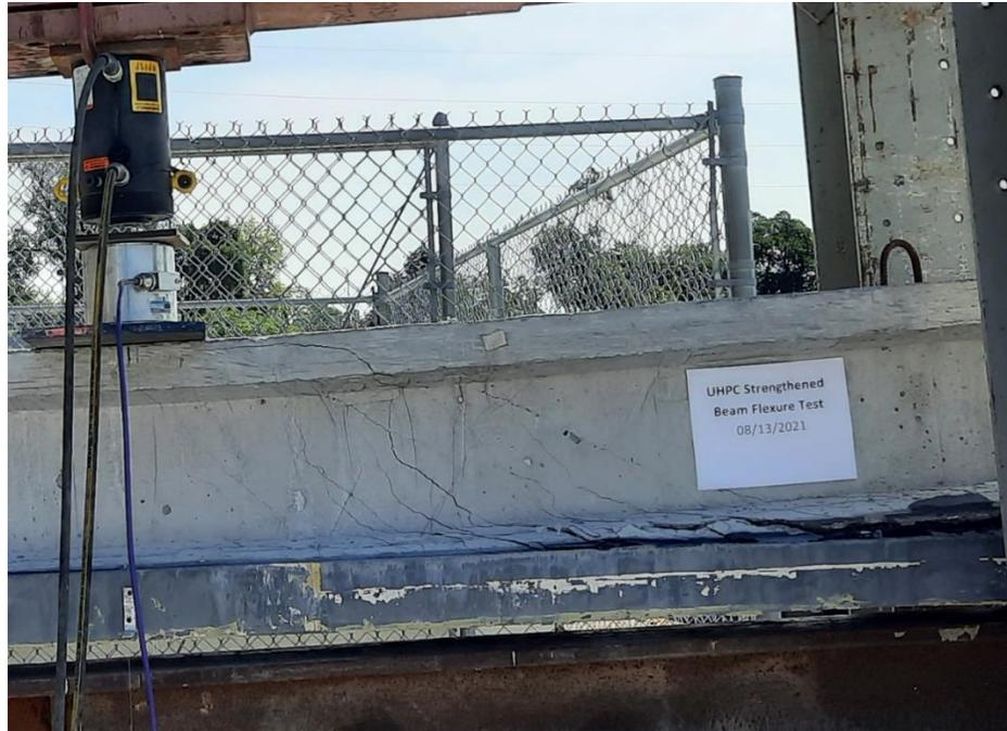
Figure 117: Strengthened beam #2 failure mode
