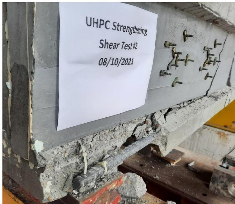
Figure 147: Strengthened beam #1 – test #2 failure mode and bar slippage in the CC beam
