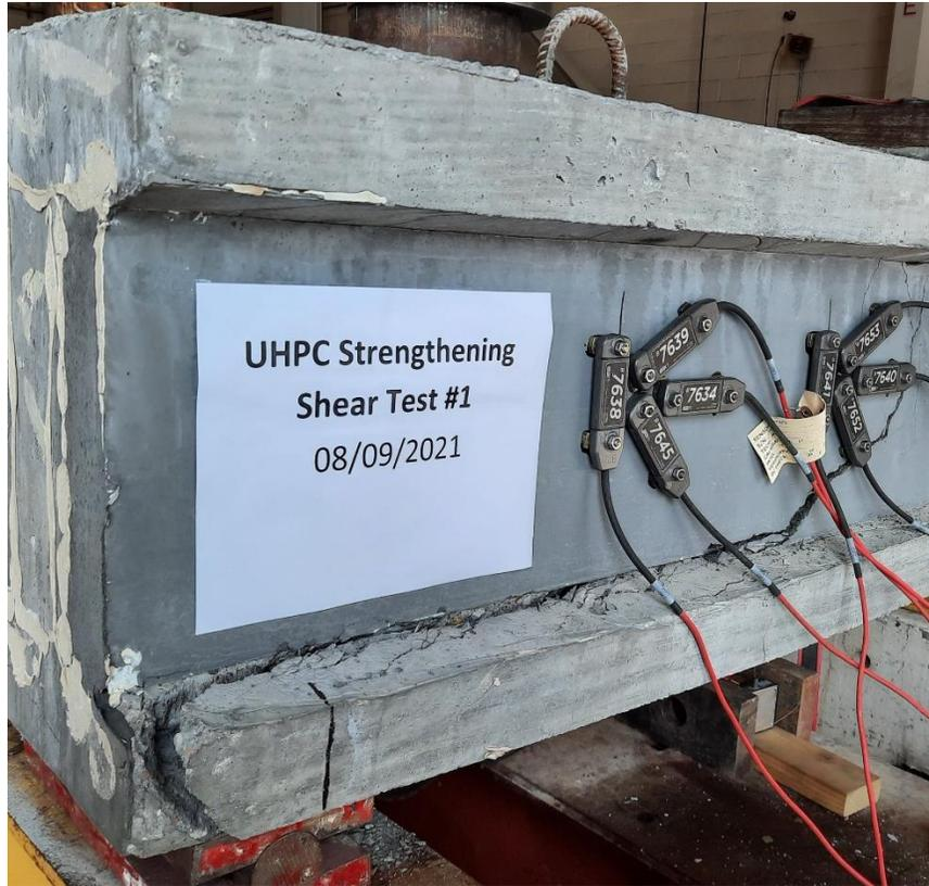
Figure 146: Strengthened beam #1 – test #1 bar slippage in the CC beam
