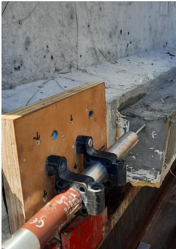
Figure 112: measuring relative displacement between CC and UHPC in strengthened beam #1
