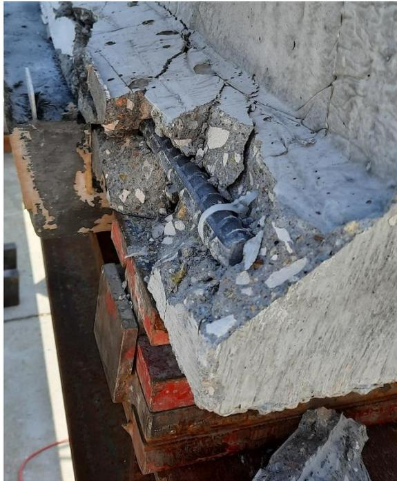
Figure 115: Strengthened beam #1 failure mode, slippage of CC tension reinforcement
