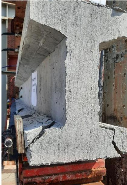
Figure 118: Strengthened beam #2 failure mode, CC tension reinforcement slippage
