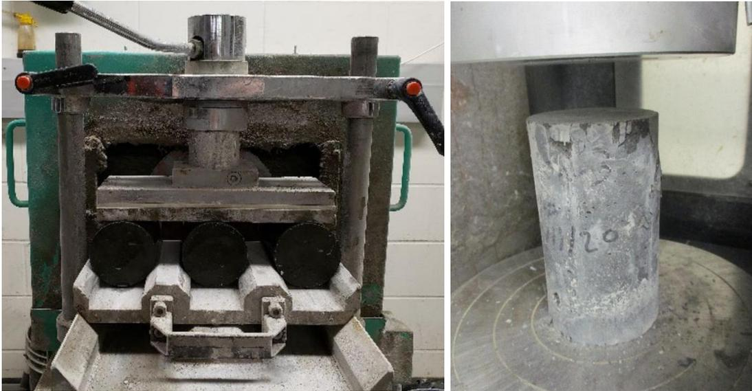
Figure 54: End grinding of UHPC cylinders (left), failed cylinder after compressive strength testing (right)
