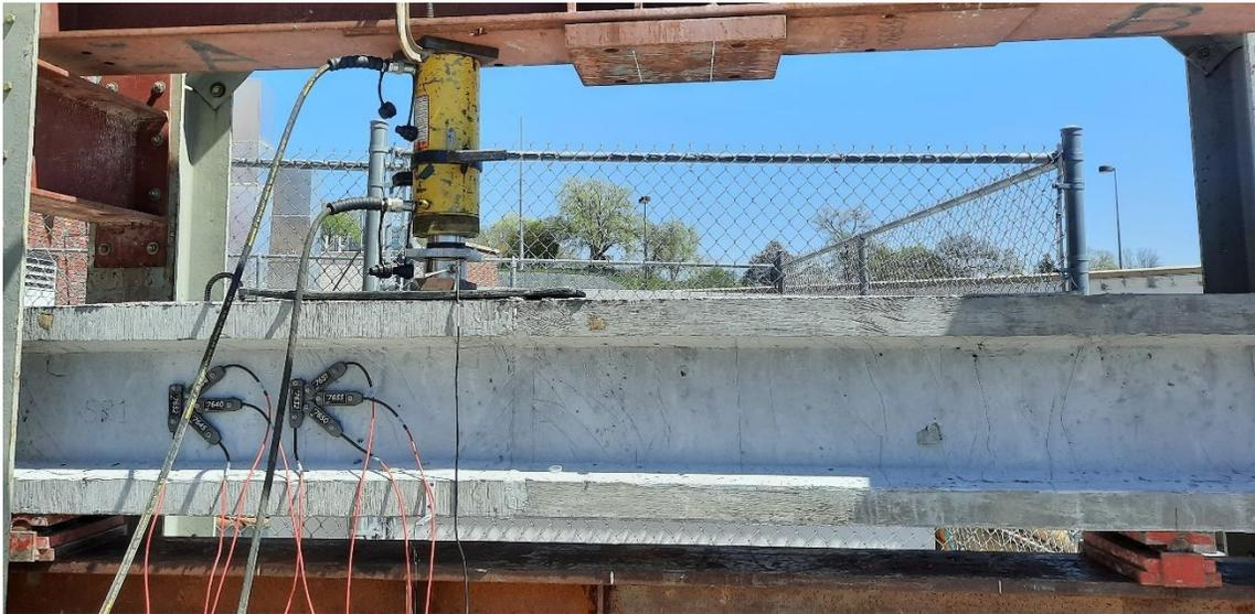
Figure 139: Reference beam test setup and instrumentation
