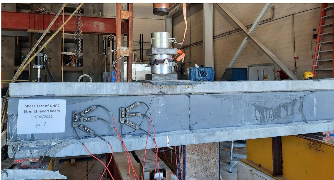
Figure 150: Strengthened beam #2 – test #2, test setup and failure mode
