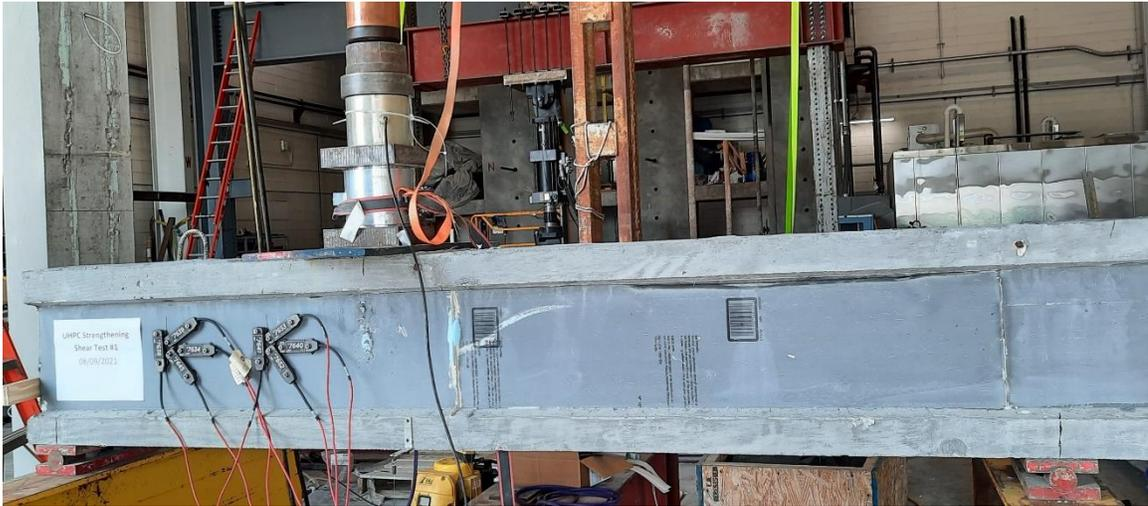
Figure 142: Strengthened beam #1 – test #1, test setup and instrumentation
