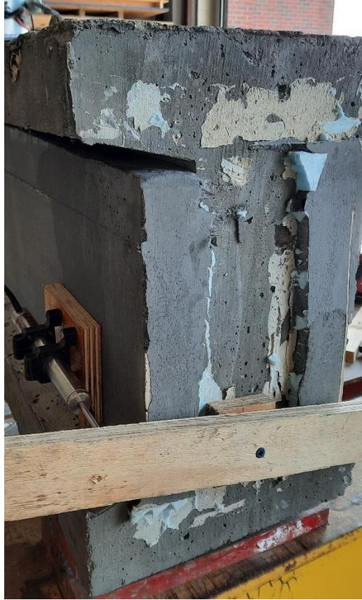
Figure 143: Measuring relative displacement between CC and UHPC in strengthened beam #1 – test #1
