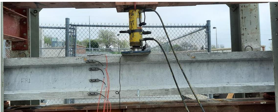
Figure 108: Reference beam test setup and instrumentation
