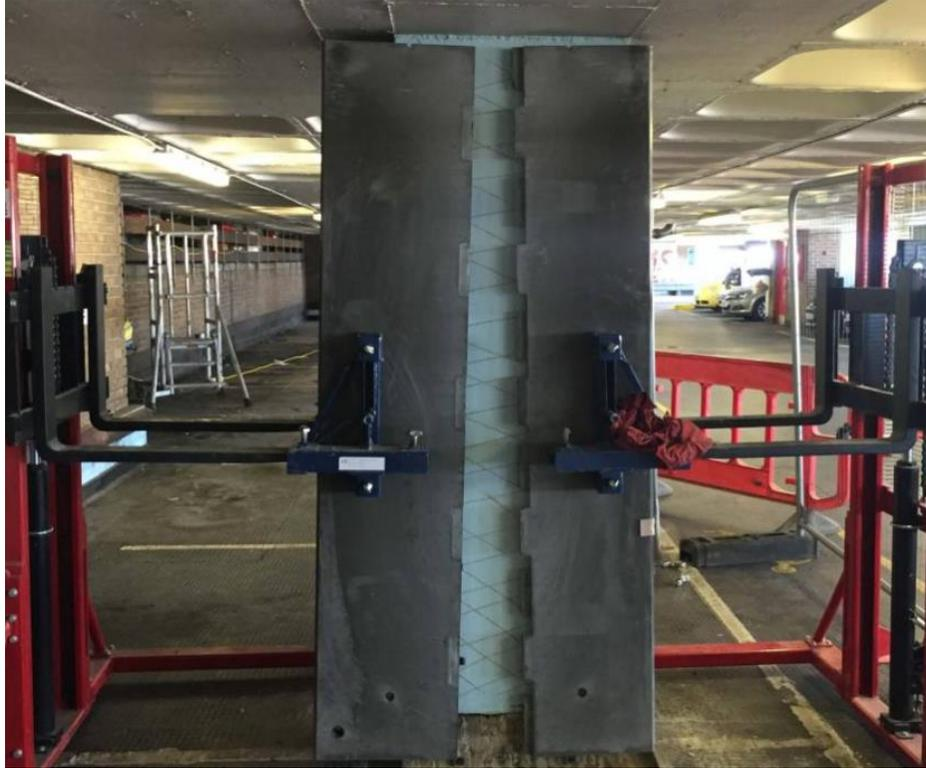
Figure 15: Precast UHPC column encasement, courtesy of Ductal website
