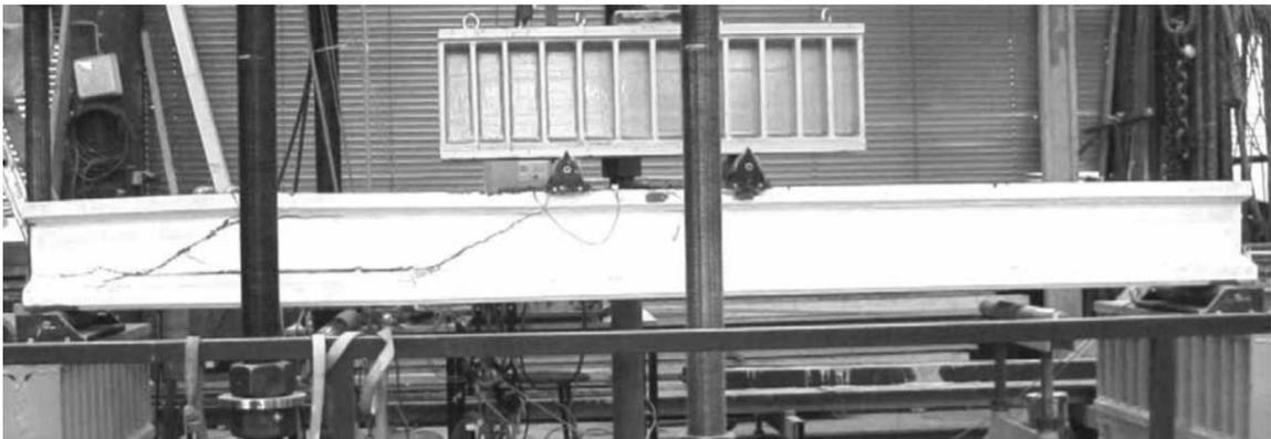
Figure 33: Shear failure mode, courtesy of Hegger et al., 2004
