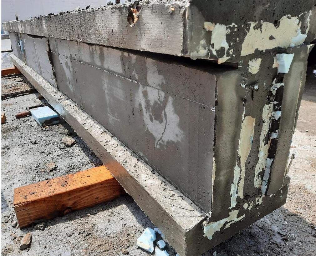
Figure 136: Poor consolidation in strengthened beam #1
