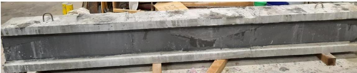
Figure 138: Casting UHPC at the poorly consolidated locations in strengthened beam #2
