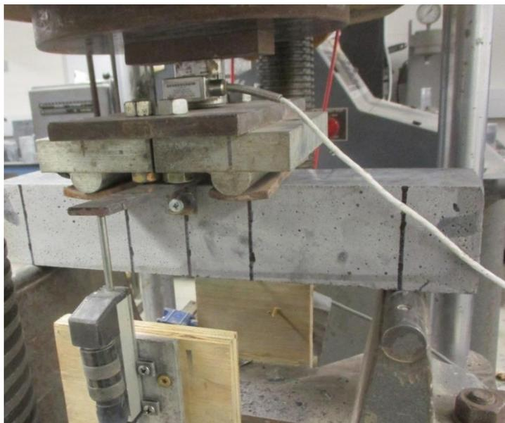
Figure 63: Flexural testing of UHPC prism
