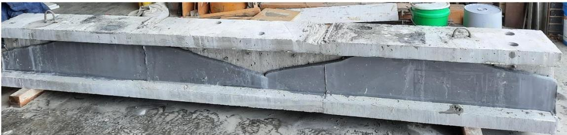
Figure 137: Poor consolidation in strengthened beam #2
