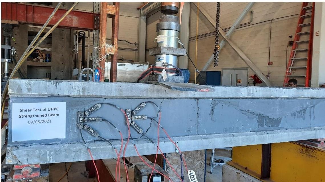
Figure 149: Strengthened beam #2 – test #1, test setup and failure mode
