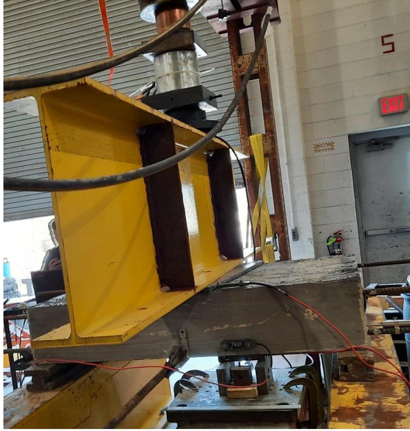
Figure 81: Test setup of the ribbed slab
