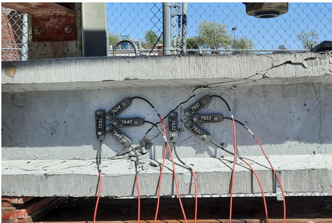
Figure 141: Reference beam failure mode
