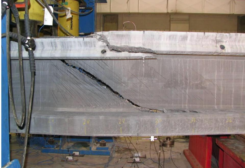
Figure 37: Shear failure mode, courtesy of Graybeal, 2009
