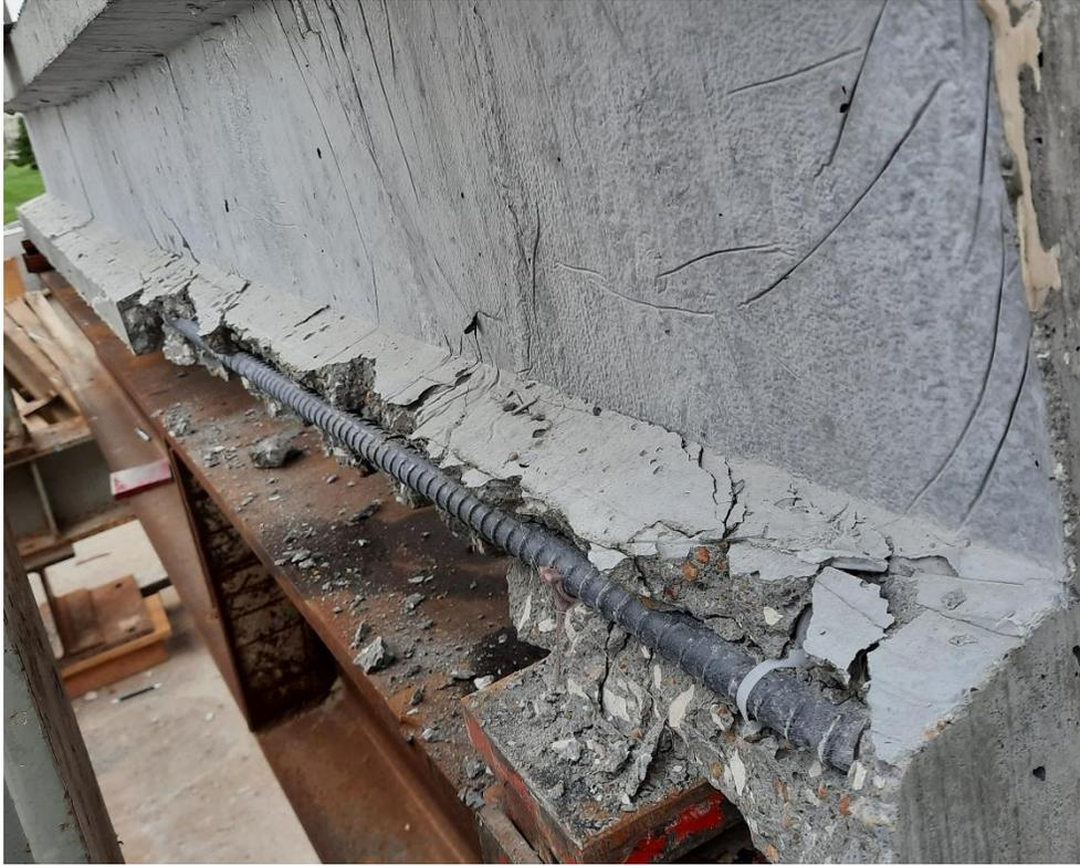
Figure 110: Reference beam failure mode
