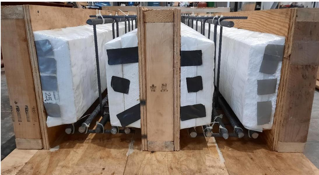
Figure 130: Formwork and reinforcement of two CC beams
