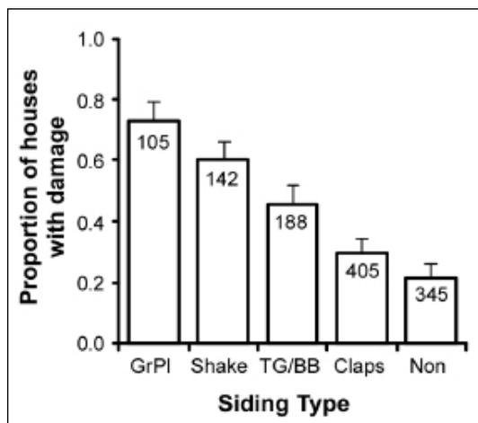
**Figure 2.** Proportion of houses near Ithaca, New York, April 2001 to March 2002, with woodpecker damage for each siding type (least-squares mean proportion and standard error after correcting for other house variables). GrPI = grooved plywood. TG/BB = tongue-and-groove and board-and-batten (pooled categories). Shake = natural and resawn shakes (pooled categories). Claps = natural and hardwood clapboards (pooled categories). Non = nonwood.
