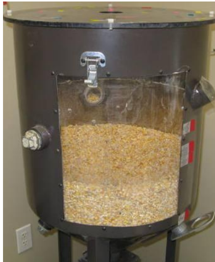
Figure 5.30 Model silo used for validation.
