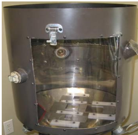
Figure 5.33 Discharge mechanisms at the bottom of the model.
