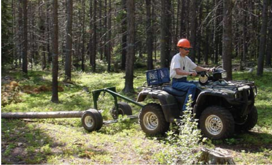
Figure 25. Cut trees can be removed from site using relatively simple technology such as this ATV and skidding arch. Photo credit: Wayne Shepperd.
