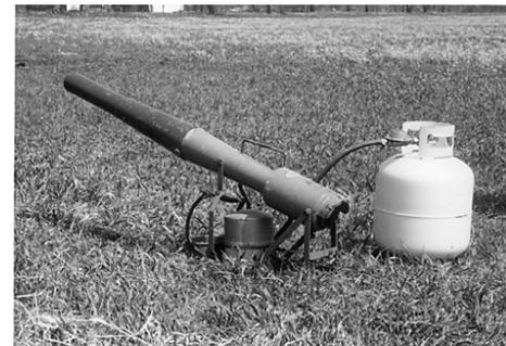
Propane exploders frighten starlings from many damage situations by producing a loud report at pre-determined intervals. For best results, exploders should be elevated above vegetation and the location and report interval changed regularly. Although these have been used successfully at some cattle feedlots, the loud noise may frighten some livestock.
