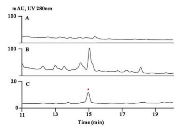
**Fig. 3.** HPLC analysis of metabolites in strains of *Lysobacter enzymogenes* OH11. A: ACL6 inframe deletion mutant; B: The ACL6 mutant supplemented with (*R*)-3-hydroxy-7-methyloctanoic acyl-SNAC; C: WAP-8294A2 standard.
