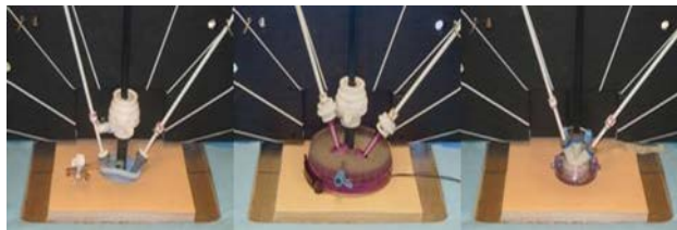
Figure 10 – Port & Insert Behavior under Moderate Instrument Articulation
