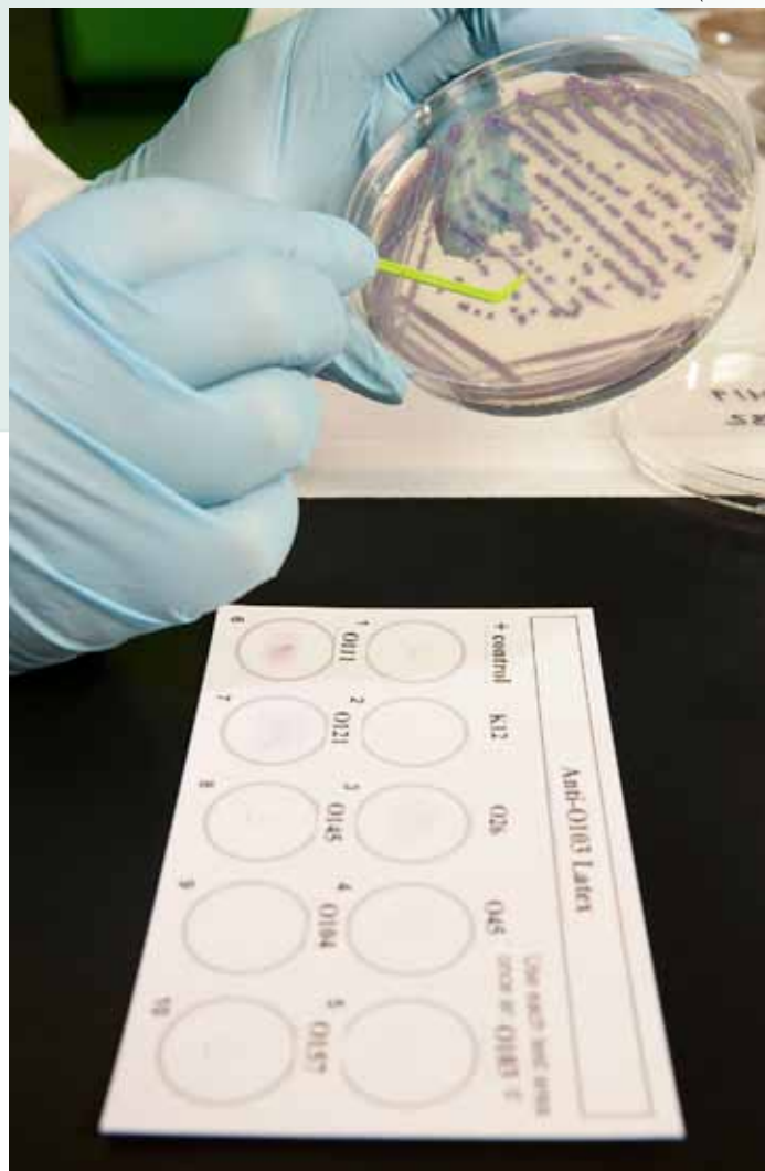
Six different serogroups of Shiga-toxin producing E. coli can be detected on this test card. A sample is placed on each test area on the card, followed by a drop of latex chemical agent bound to a specific antibody for that serogroup. The results are visible within a few minutes.
