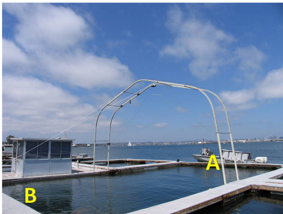
Fig. 1. Picture of the test enclosure with station locations designated by yellow letters. The arch over the enclosure held the overhead video cameras. Dolphins initiated each trial sequence on the middle of the right side of the pen (station A), swam across the pen and touched a paddle on the opposite side (station B), and then returned to the starting location. The sound source was 1 m behind station B and 1 m below the surface. During exposure trials, dolphins were exposed to the simulated sonar signal at the midpoint of the enclosure.
