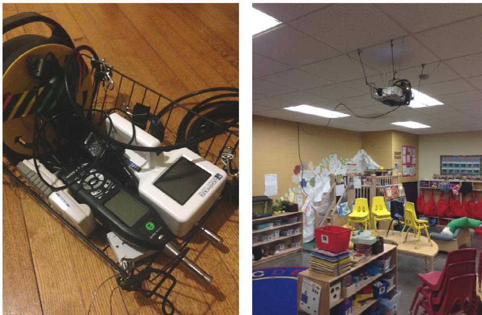
Illuminance was measured at four locations in each classroom relative to luminaires, according to *Standard Measurement and Verification Plan for Lighting Retrofit Projects for Buildings and Building Sites* (Richman, 2012). Taken at night after lamps had reached steady output, the two largest illuminance values were averaged for each classroom. The ratio of the largest to smallest illuminance values created the
