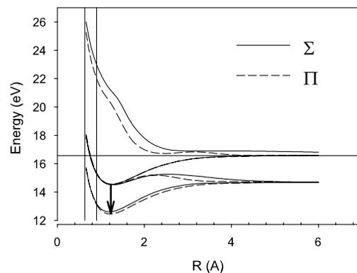
FIG. 2. Potential energy curves of  $\text{H}_2$  triplet states leading to  $\text{H}(n = 2, 3)$  states. The Frank-Condon region lies between the vertical lines; the horizontal line is the threshold for  $\text{H}(1s) + \text{H}(3s)$ : 16.57 eV. The vertical arrow indicates the molecular transitions we observe.
