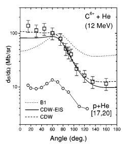
FIG. 5. The angular distributions of single-differential cross sections for  $C^{6+}$  + He (1 MeV/u,  $v_p$ =6.35). The different calculations are also shown by solid (CDW-EIS model), dashed (CDW model), and dotted (B1 model) lines. The circles joined by lines represent the SDCS for p + He at the same projectile velocity, and are taken from Refs. [17,20].
