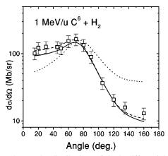
FIG. 6. The angular distributions of single-differential cross sections for  $\rm H_2$  targets. The different calculations are also shown by solid (CDW-EIS model), dashed (CDW model), and dotted (B1 model) lines.
