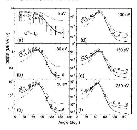
FIG. 4. The angular distributions of electron DDCS's for 1-MeV/u  $C^{6+}+H_2$  measured at different electron energies as indicated in different panels. The different calculations are also shown by solid (CDW-EIS model), dashed (CDW model), and dotted (B1 model) lines.
