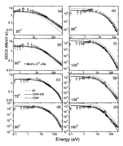
FIG. 1. The double-differential cross sections of electron emission for a He target. The data in different panels correspond to different emission angles as indicated. The CDW-EIS (solid line), CDW (dashed line), and B1 (dotted line) calculations are also shown.
