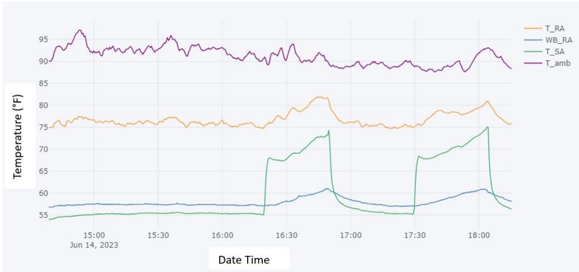
Figure 29: Temperatures in return, supply, and ambient air
