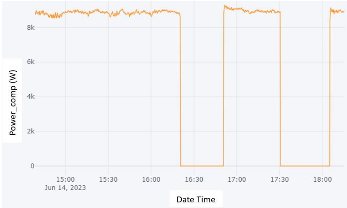
Figure 33: Logged compressor power (considering a power factor of 0.95)
