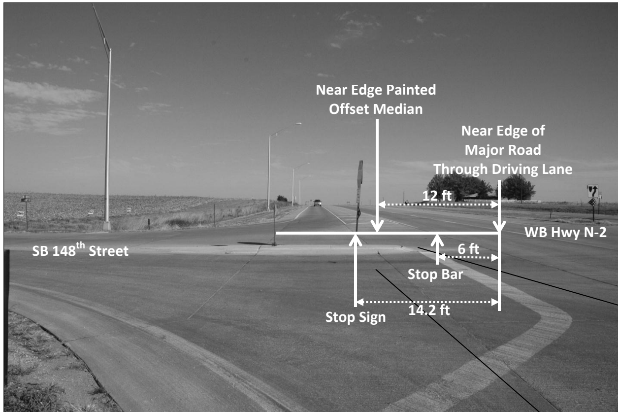
Figure 2.14 Lateral Dimensions to Key Cues for Driver Positioning at Southbound Minor Road Stop-Controlled Approach of Site 1, 148 th Street & Hwy N-2
