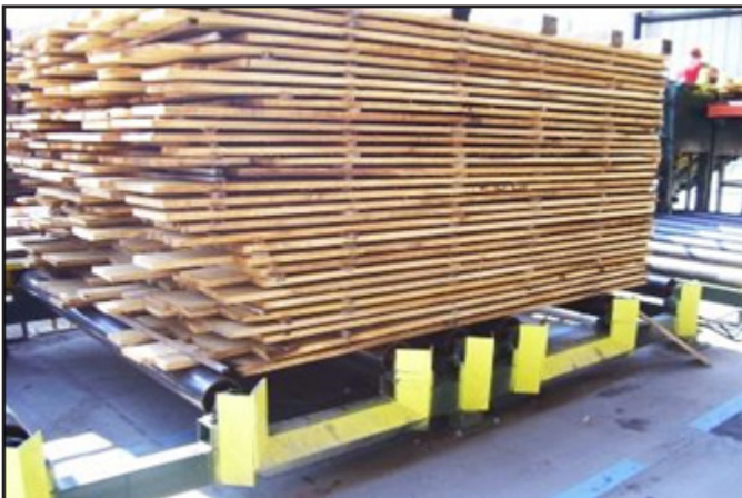
The practice of even-end piling is generally not recommended (Photo by Travis Allen).
