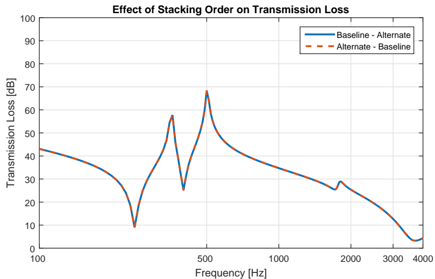
Figure 5.19: TL of double layer with different stacking order. Baseline then alternate configuration (solid), alternate then baseline configuration (dashed)
