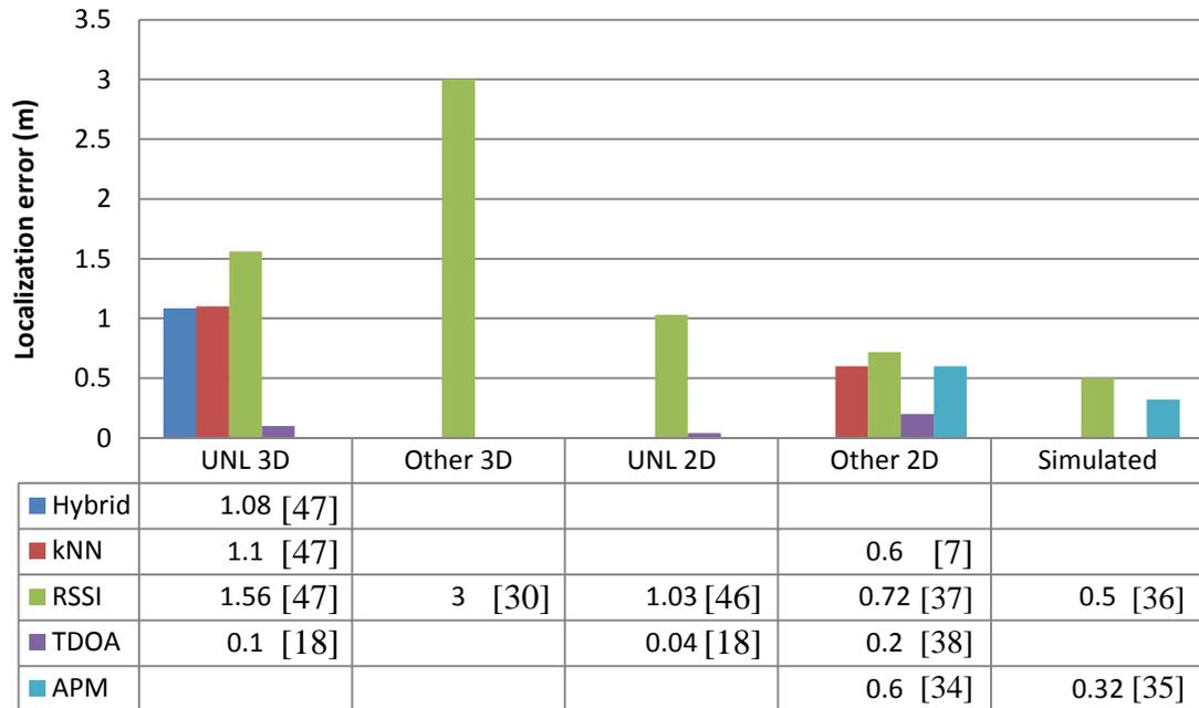
**Figure 5-8: Localization error comparison**
