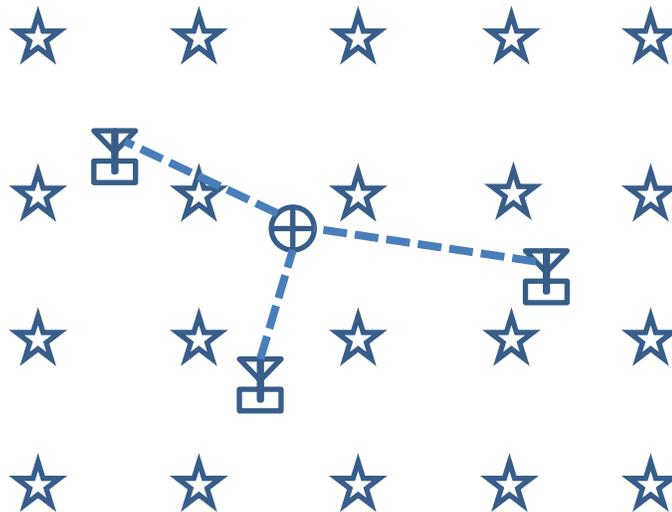
**Figure 2-5: RSSI with fingerprinting**
