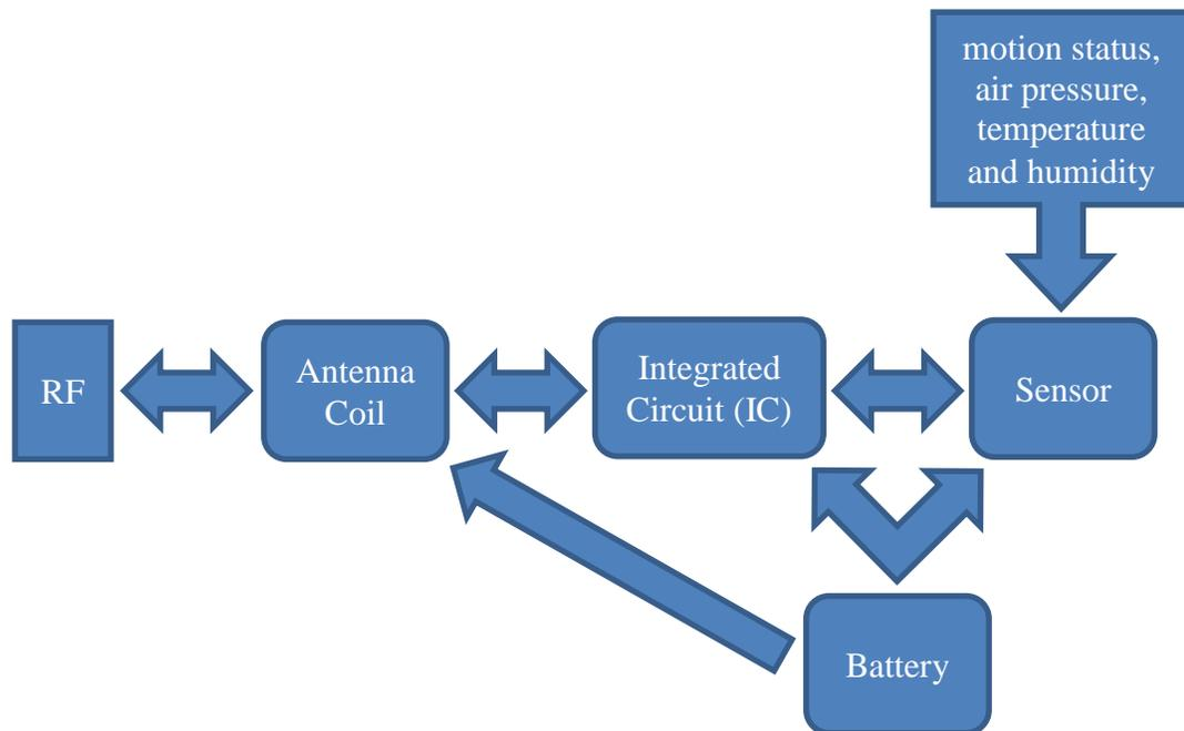
**Figure 2-3: Active RFID tag structure**
