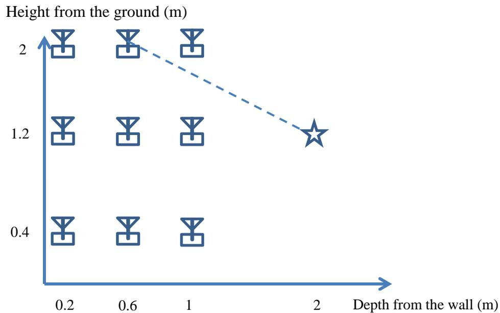
**Figure 4-1: Layout scheme of reader test**
