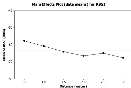
(a) signal strength (mean) versus distance
