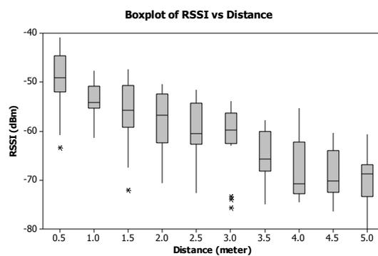
(c) signal strength versus distance using boxplot
