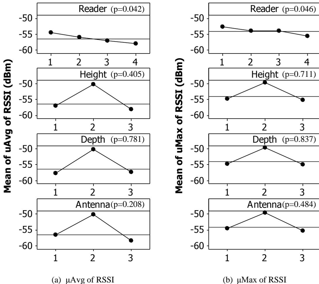
Figure 5-1: Main effects plot for reader test
