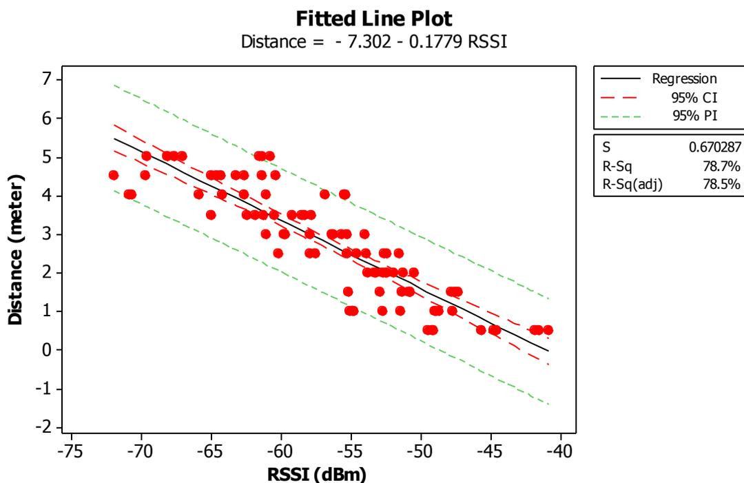
Figure 5-11: Linear regression of ranging test (battery-assisted passive system)
