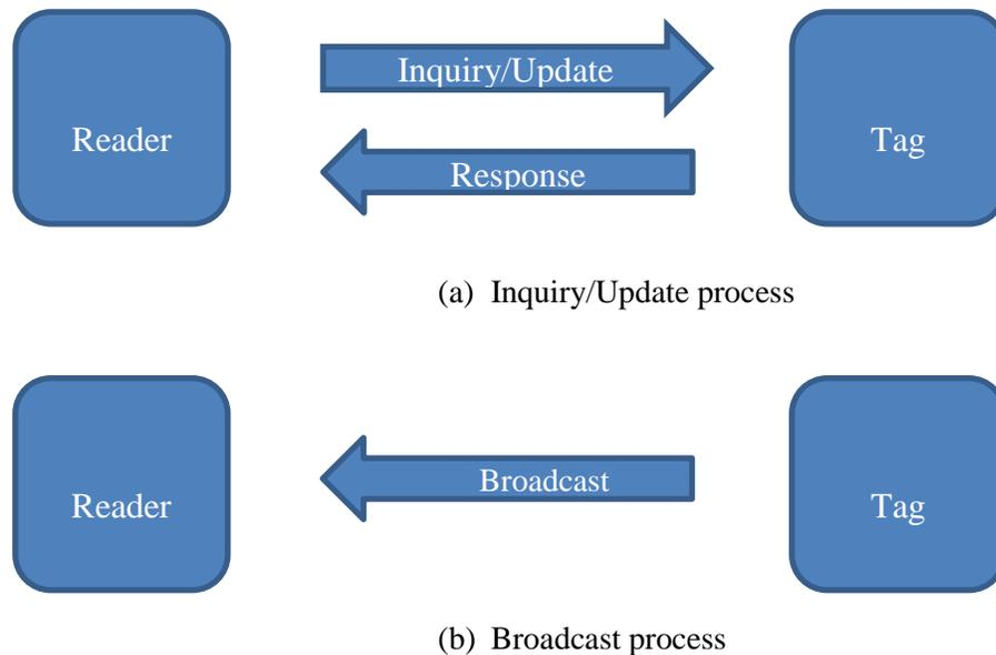
**Figure 2-2: Communication models between RFID tags and readers**
