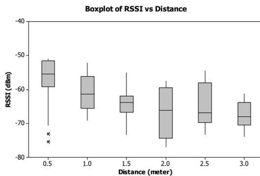
(c) signal strength versus distance using boxplot
