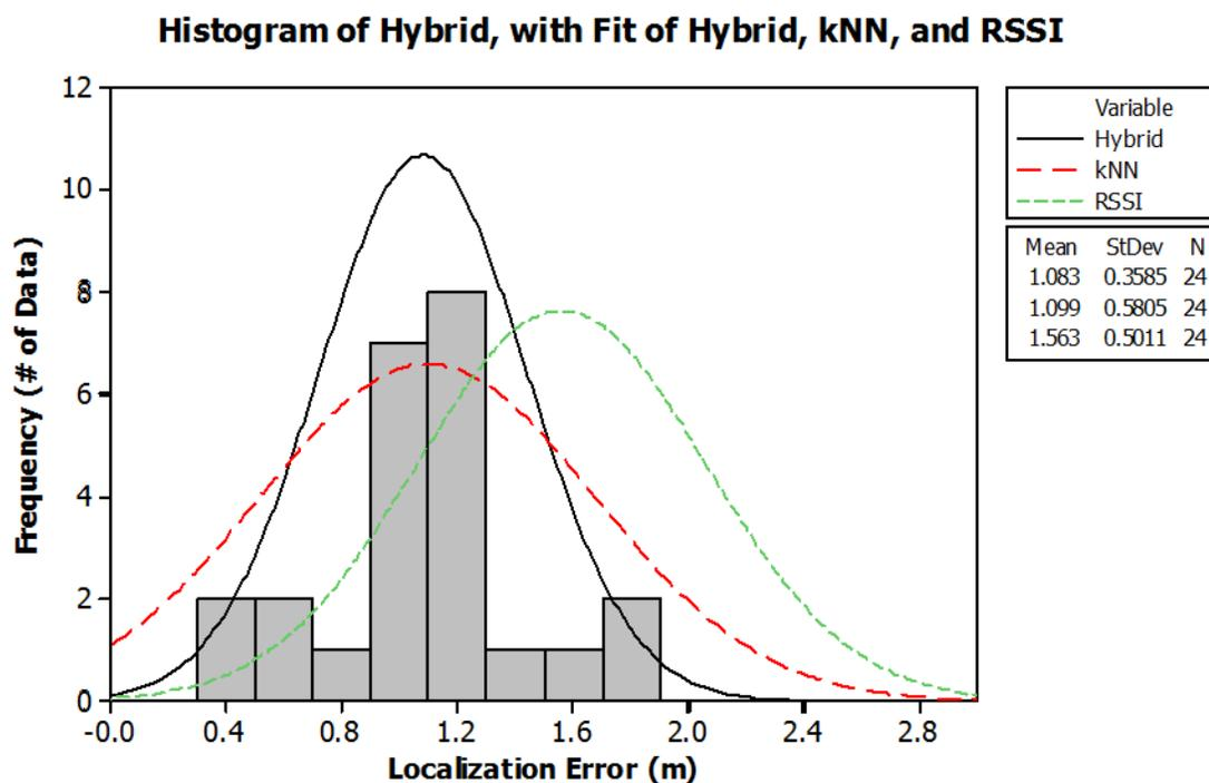
Figure 5-7: Localization error histogram with fit
