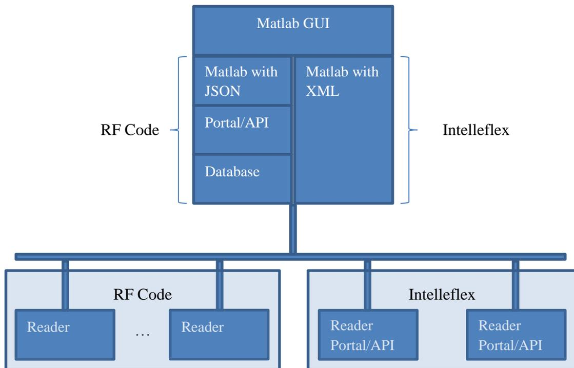
**Figure 4-15: Network and software structure of both systems**
