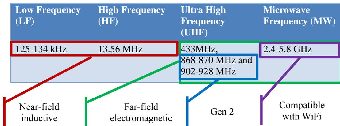
Figure 2-1: Typical frequency bands used for RFID
