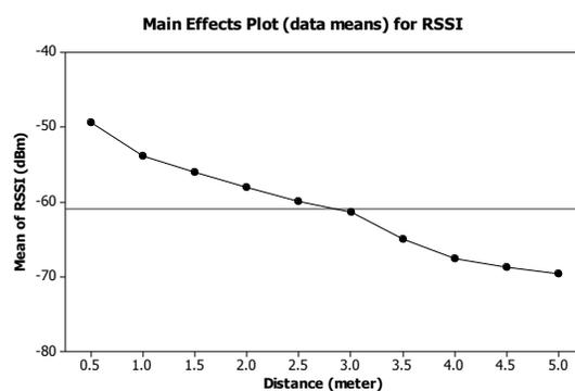
(a) signal strength (mean) versus distance
