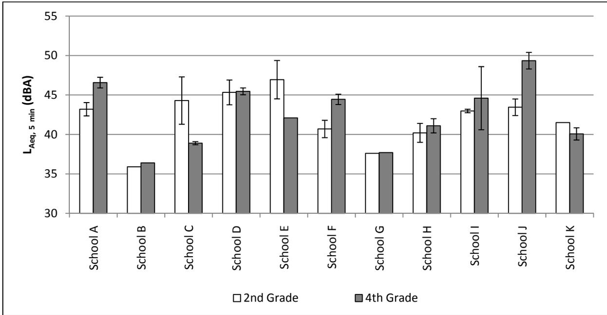
**Figure 2A**—weighted equivalent sound levels for 11 of the schools, all with consistent mechanical system conditions for the BNL measurements (BNL measured with central mechanical system activated). The bars show the range in BNL about the average value for all classrooms at each grade level in each school.
