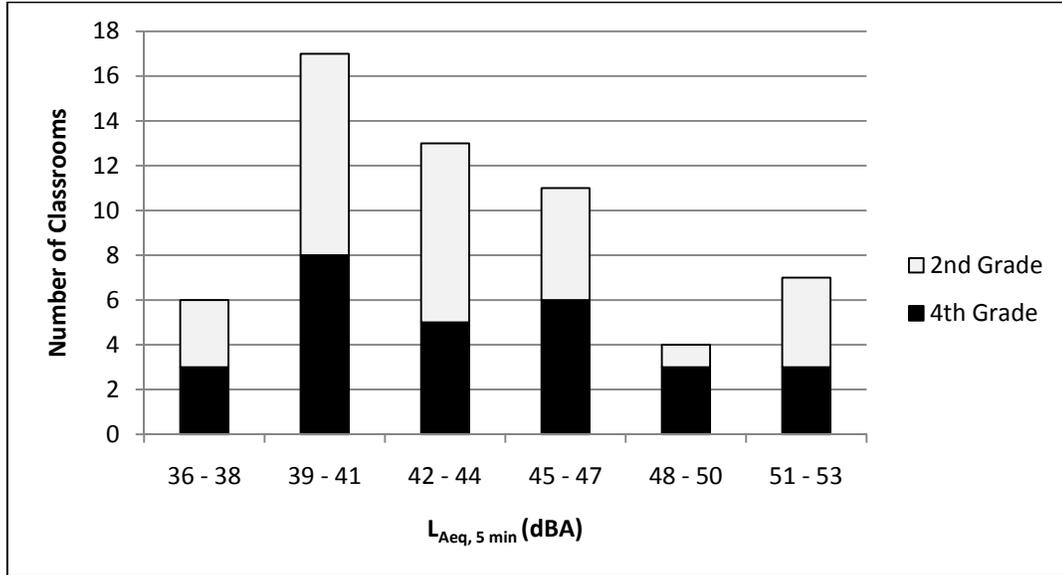
**Figure 1** A-weighted equivalent sound levels for all of the classrooms measured. This includes spaces with the BNL measured with central mechanical system activated (50 classrooms), with the central mechanical system deactivated (2 classrooms), and with the window air-conditioning units activated when present (6 classrooms).
