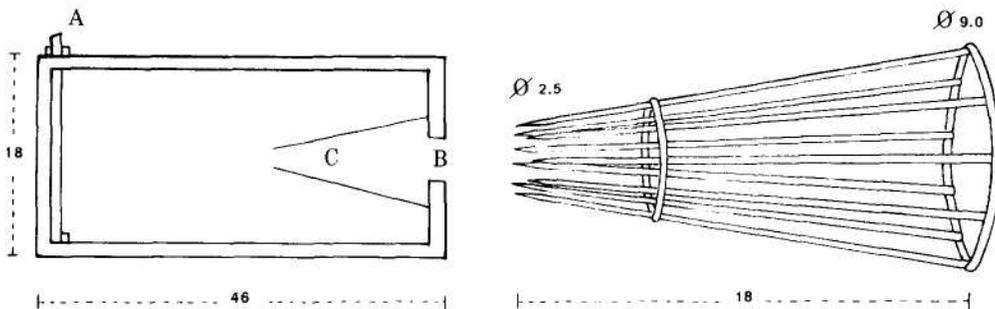
Figure 2. Left: longitudinal schematic section of an artificial nest for dormouse capture; A, sliding closure for specimen removal; B, circular entry hole (Ø 6); C, device preventing animal from re-exit. Right: detailed drawing of the same device as in C. All reported dimensions are in cm.
