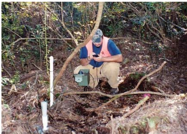
Technician Justin Bennett conducting maintenance and downloading of soil moisture and ground water well monitoring equipment (Dare County, NC). Credit: Roberta Bartlette.
