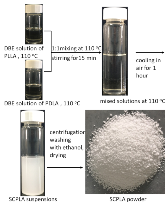
Scheme 1. Preparation Process of the SCPLA
