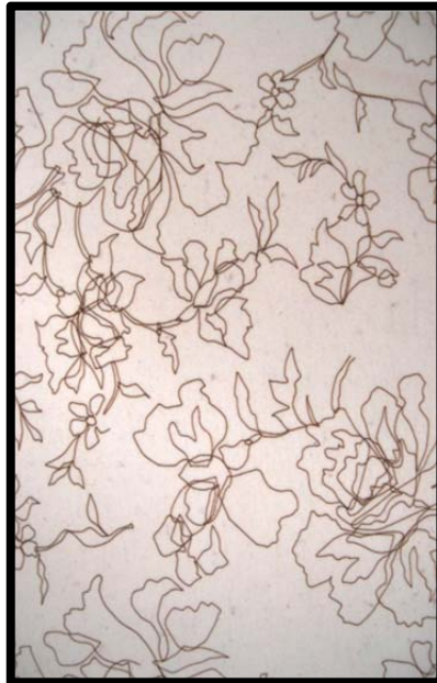
Figure 7, left. Vector cut into the surface of industrial felt.
