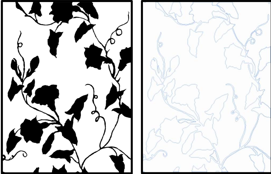
Figure 3, left. A black and white design for a Raster setting Figure 4, right. A blue linear design for a Vector cut. Images and designs by author. Copyright 2010 Jessica Payne
