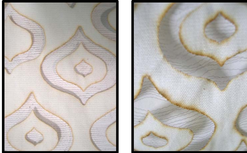
Figure 11. Raster cut through a woven cotton textile with a weft inserted fine metal weft thread. Images by author. Copyright 2010 Jessica Payne
