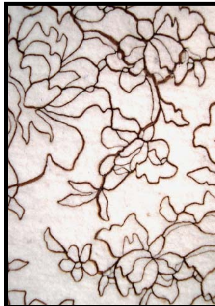
Figure 7, left. Vector cut into the surface of industrial felt.
