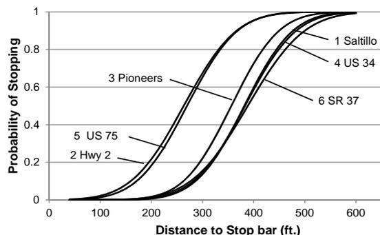
Fig. 3 - Critical distances along probability of stopping curve
