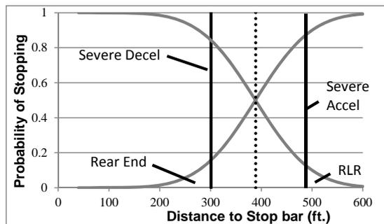
Fig. 1 - Critical distances along probability of stopping curve
