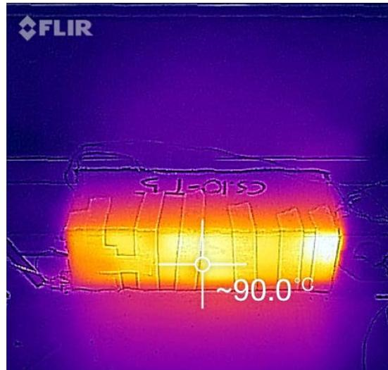
**Figure 3-11: Infrared image of uncovered CSEB during heating**
