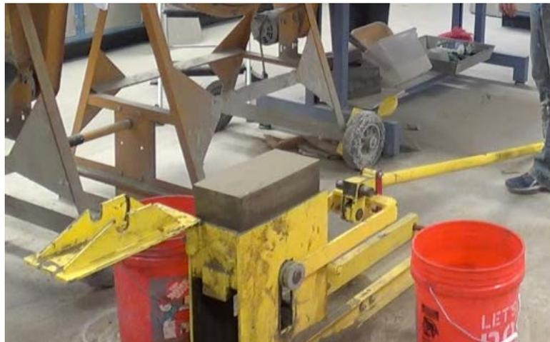
**Figure 3-3: Finished CSEB after block press**
