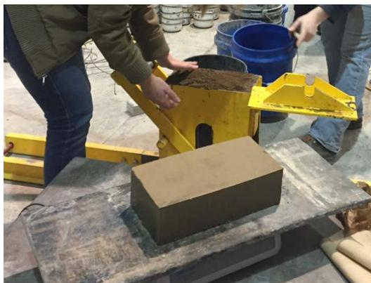
**Figure 4-3: CSEB fabricated at University of Nebraska- Lincoln**
