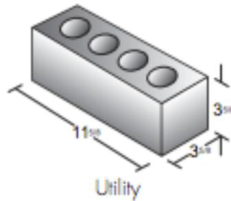
**Figure 4-4: Typical Clay brick used in this study**
