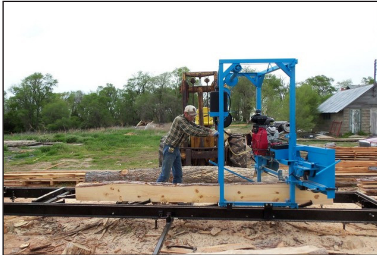
Jeff Carpenter processing a log using the EZ Boardwalk 40 portable band saw mill.
