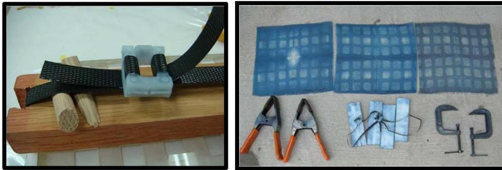
**Figure 5, left.** Alternative non-metal tie up with polypropylene strapping tape, plastic buckle and wood wedges.
