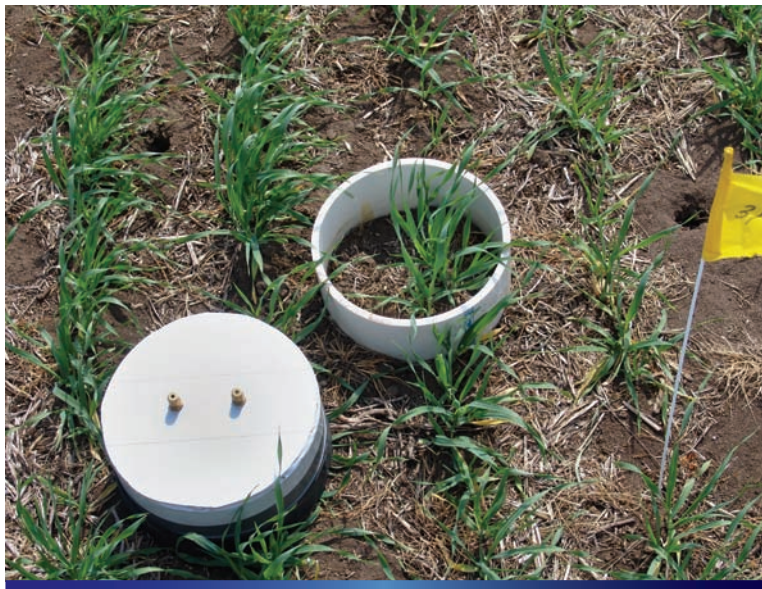
Close-up of a static chamber in a field of malt barley. The chamber is used to collect greenhouse gas samples coming off this tiny section of the plot.
