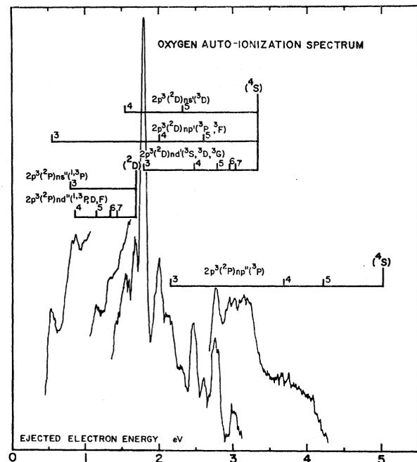
FIG. 2. Energy spectrum of electrons from oxygen gas bombarded by 100-keV  $H^+$  or  $He^+$  ions. Six series are seen; four representing auto-ionizing transitions into the  ${}^4S$  continuum and two into the  ${}^2D$  continuum. Resolution 70 meV.
