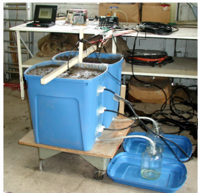
Figure 3. Laboratory lysimeter setup.
