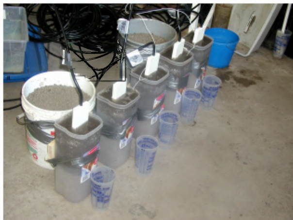
Figure 2. Performing soil TDR experiments in the laboratory.
