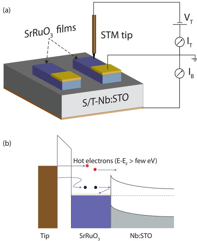
FIG. 2. (a) Fabrication of multiple SrRuO<sub>3</sub> devices grown on Nb:STO. Analyses were done on many different devices to understand the electronic behavior of the film-substrate interface. (b) Schematic diagram of BEEM, where the Pt-Ir STM tip injects hot electrons over the vacuum barrier into a thin metallic film of SrRuO<sub>3</sub>. The transmitted electrons that satisfy the energy and momentum criteria to overcome the SBH at the interface are collected in the Nb:STO semiconductor.
