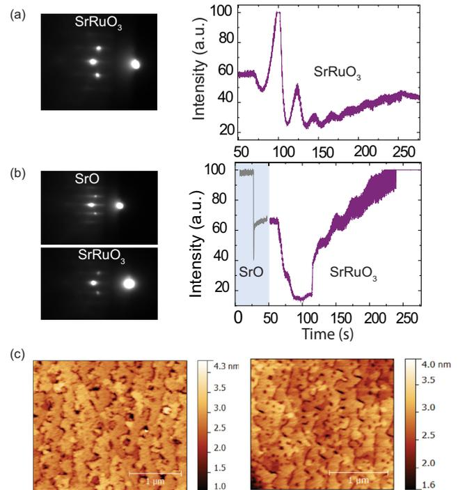
FIG. 1. Growth of 8 u.c. of SrRuO<sub>3</sub> on TiO<sub>2</sub> and SrO terminated substrates. (a) RHEED data for SrRuO<sub>3</sub> growth on nonengineered substrate T-Nb:STO. (b) RHEED data for the growth of a monolayer of SrO followed by 8 u.c. of SrRuO<sub>3</sub>. (c) AFM scan image of T-Nb:STO and S-Nb:STO.
