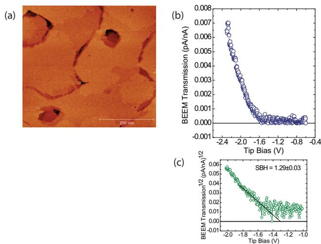
FIG. 4. (a) STM topography of 8 u.c. of SrRuO<sub>3</sub> grown on S-Nb:STO at  $V_{\text{tip}} = -1.4$  V and  $I_{\text{tunnel}} = 4$  nA. (b) Corresponding BEEM spectra through 8 u.c. of SrRuO<sub>3</sub> grown on S-Nb:STO. (c) The extracted local Schottky barrier height. Clearly, the local SBH matches with that extracted from SrRuO<sub>3</sub> grown inside the trenches of T-Nb:STO as shown in Fig. 3(b).
