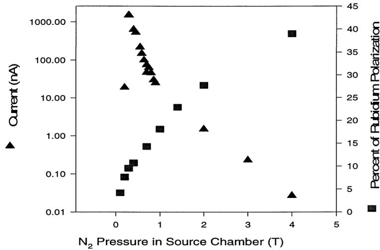
Figure 3: Current and Rubidium Polarization vs Nitrogen Pressure
