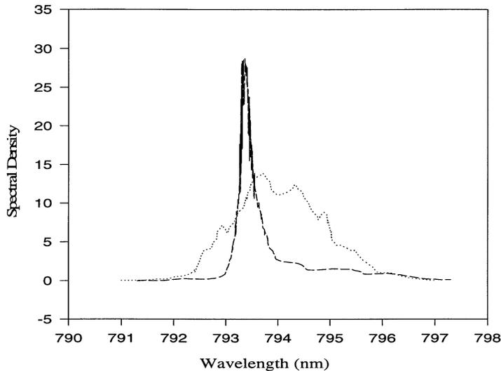
Figure 2: Narrowing with Grating Feed-back
